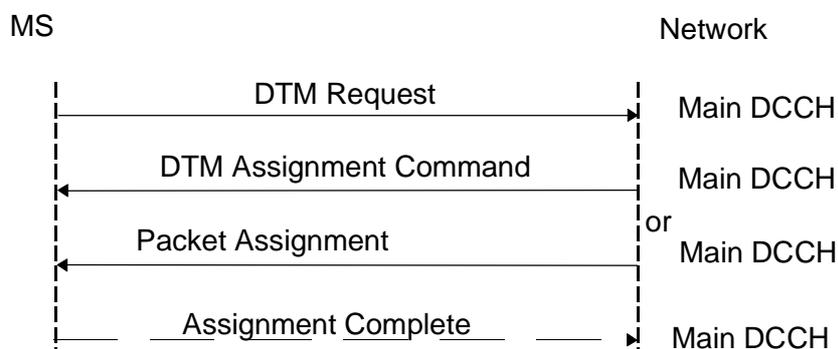
**Figure 24b: Access and allocation for the packet request procedure, uplink packet transfer**
