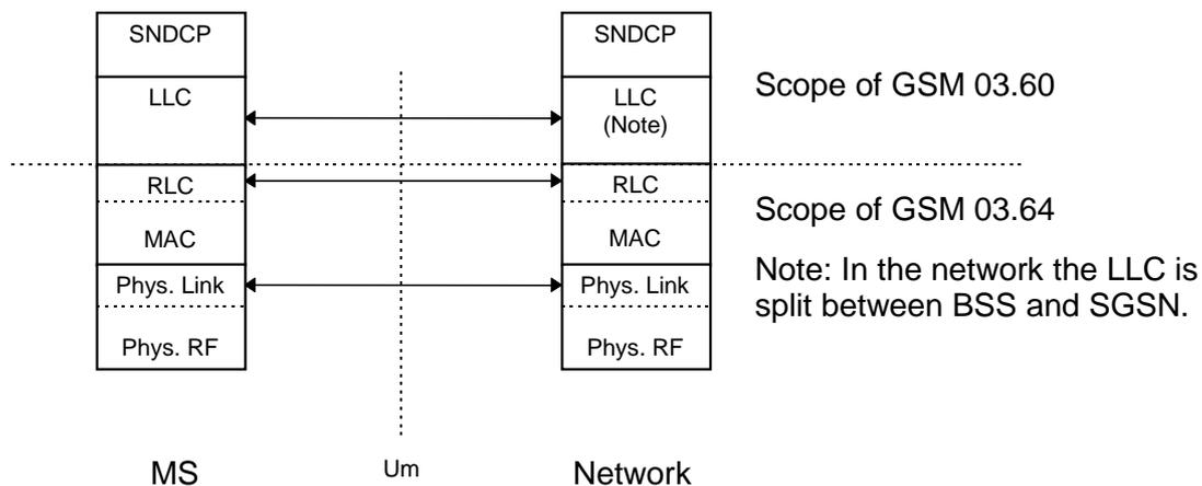
Figure 3d: GPRS MS – Network Reference Model
