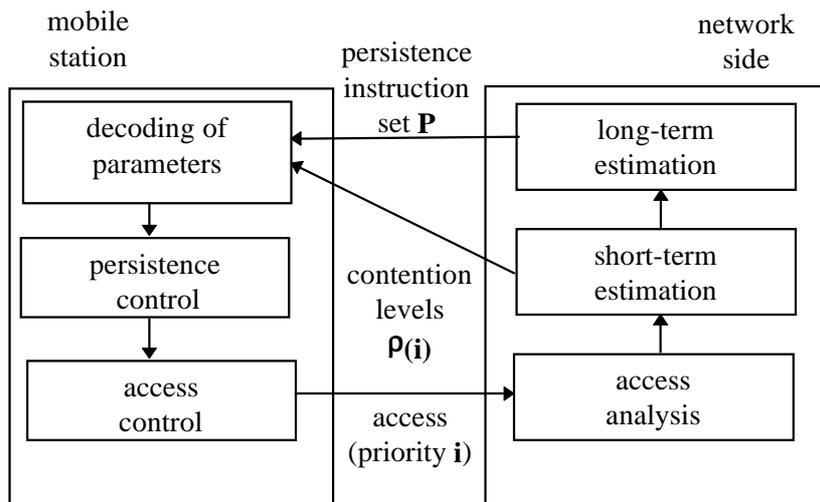
**Figure 24: Basic principle of random access traffic control**
