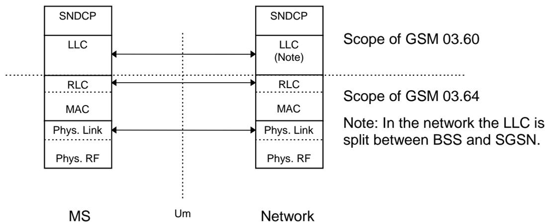
Figure 7: GPRS MS – Network Reference Model
