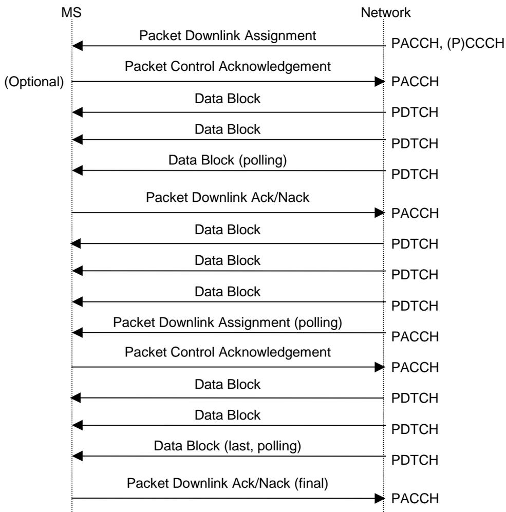
Figure 27: An example of downlink data transfer
