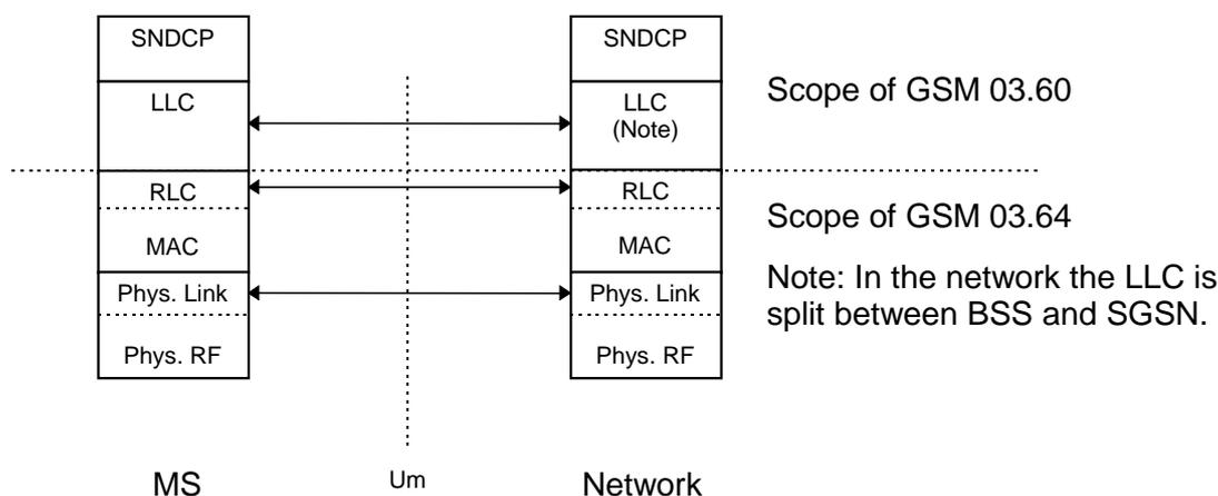
**Figure 3: GPRS MS – Network Reference Model**
