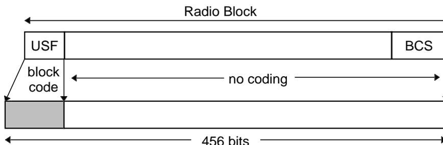
**Figure 6: Radio Block structure for CS-4**
