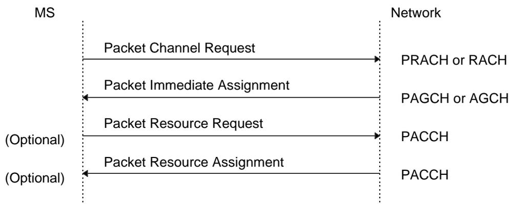
**Figure 9: Access and allocation for the one or two phase packet access, uplink packet transfer**
