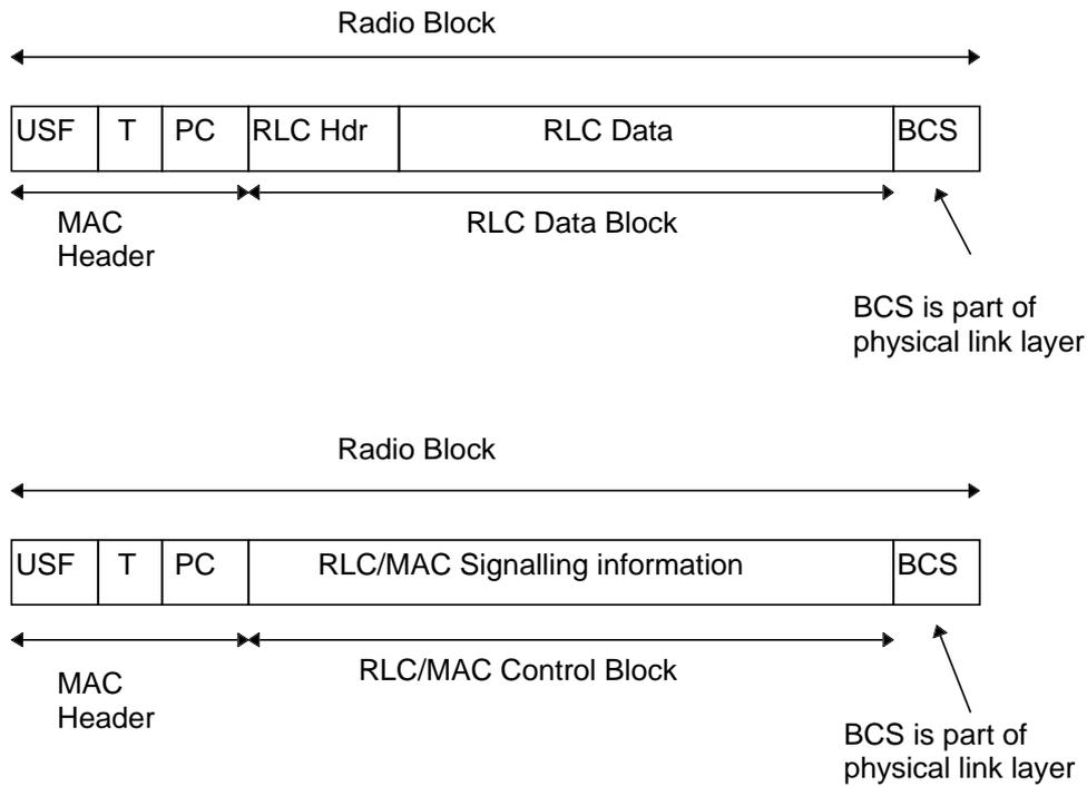
Figure 4: Radio Block structures
