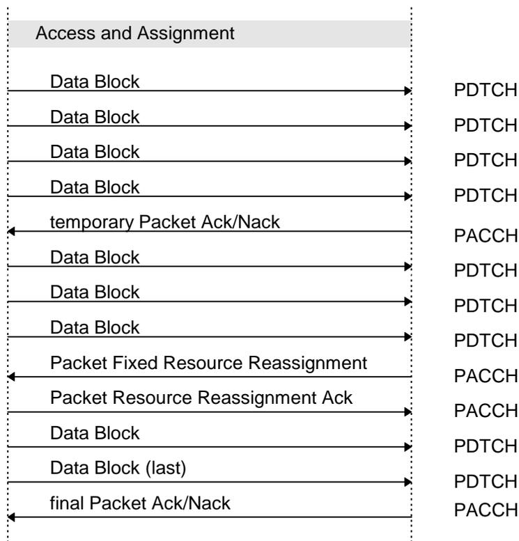
Figure 12: An example of fixed allocation uplink data transfer
