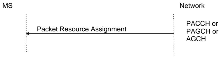
**Figure 14: Downlink PDTCH Assignment in GPRS Ready state using Packet Resource Assignment message.**
