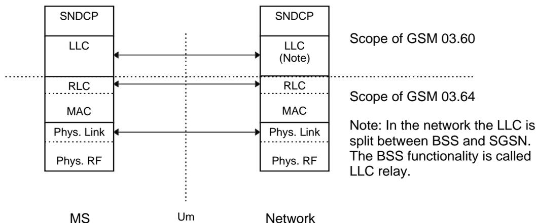
Figure 3: GPRS MS – Network Reference Model
