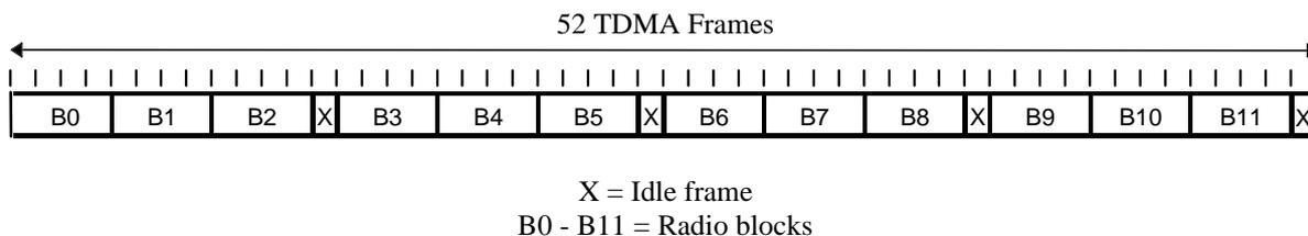
**Figure 2: Multiframe structure for PDCH**
