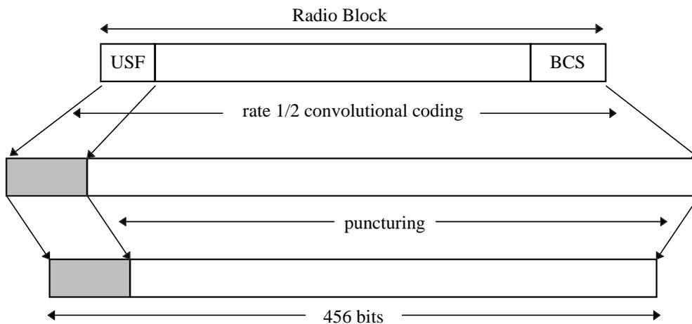
Figure 5: Radio Block structure for CS-1 to CS-3
