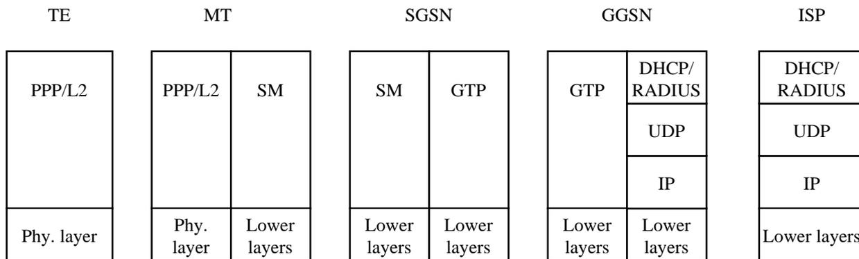
**Figure 11: Signalling plane of non transparent case**
