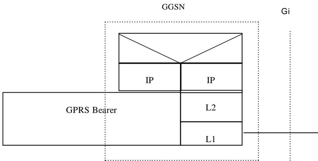
Figure 8: The protocol stacks for the GiIP reference point
