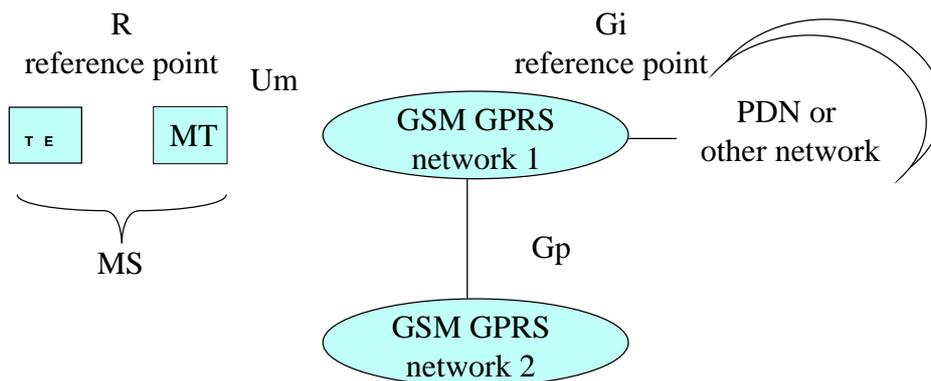
Figure 1: GPRS Access Interfaces and Reference Points
