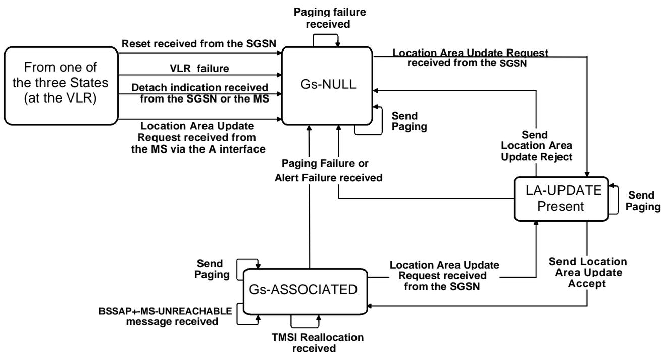
Figure 4.1/GSM 09.18: State diagram at the VLR
