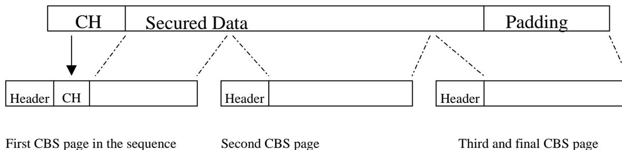
In the above figure, Header = 6 Octet header as defined in GSM 03.41 (i.e. SN, MID, DCS and PP) and CH = Command Header
