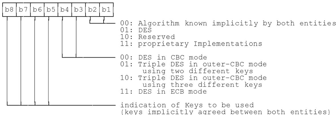
DES is the algorithm specified as DEA in ISO 8731-1 [9]. DES in CBC mode is described in ISO/IEC 10116 [10]. Triple DES in outer-CBC mode is described in section 15.2 of [20]. DES in ECB mode is described in ISO/IEC 10116 [10].
