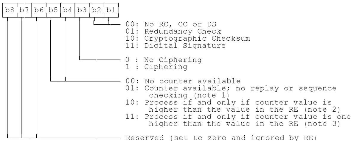
NOTE 1: In this case the counter value is used for information purposes only, (e.g. date or time stamp). If the Command Packet was successfully unpacked, the counter value can be forwarded from the Receiving Entity to the Receiving Application. This depends on proprietary implementations and happens in a application dependent way.
