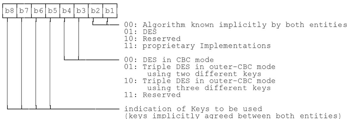
DES is the algorithm specified as DEA in ISO 8731-1 [9]. DES in CBC mode is described in ISO/IEC 10116 [10]. Triple DES in outer-CBC mode is described in section 15.2 of [20].
