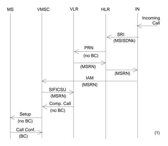
NOTE: (1) This BC is derived from information stored in the MS, according to its configuration.
