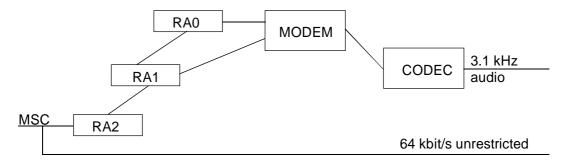
Figure 8: Protocol structure in the MSC/IWF (transparent)
