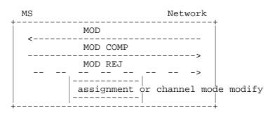
Figure 5.10b/GSM 04.08: In-call modification sequence initiated by network
