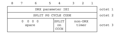
Figure 10.5.122/GSM 04.08: DRX parameter information element
