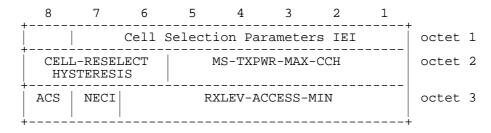
Figure 10.5.23/GSM 04.08: Cell Selection Parameters information element
