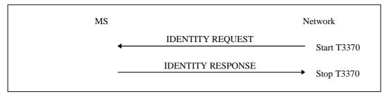
Figure 4.7.8/1 GSM 04.08: Identification procedure
