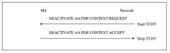
Figure 6.9/GSM 04.08: Network initiated AA PDP context deactivation procedure
