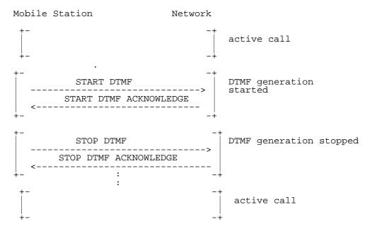
Figure 7.13/GSM 04.08: DTMF protocol control
