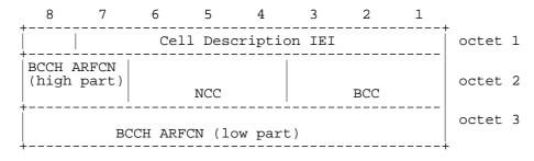
Figure 10.5.20/GSM 04.08: Cell Description information element
