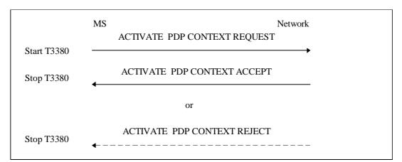
Figure 6.3/GSM 04.08: MS initiated PDP context activation procedure
