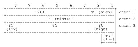
Figure 9.3/GSM 04.08: Frame synchronization information element
