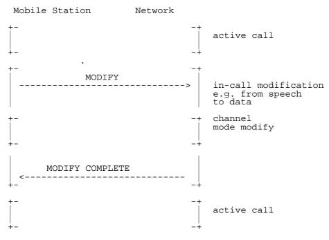
Figure 7.17/GSM 04.08: In-call modification
