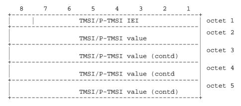
Figure 10.5.70/GSM 04.08: TMSI/P-TMSI information element
