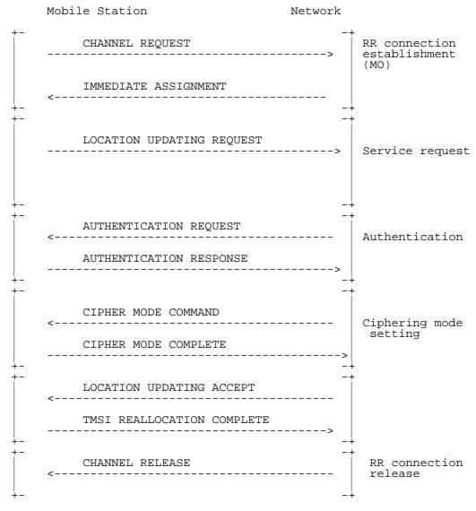
Figure 7.9/GSM 04.08: Location updating: successful case
