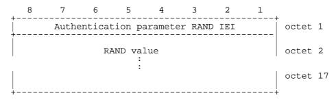
Figure 10.5.75/GSM 04.08: Authentication Parameter RAND information element
