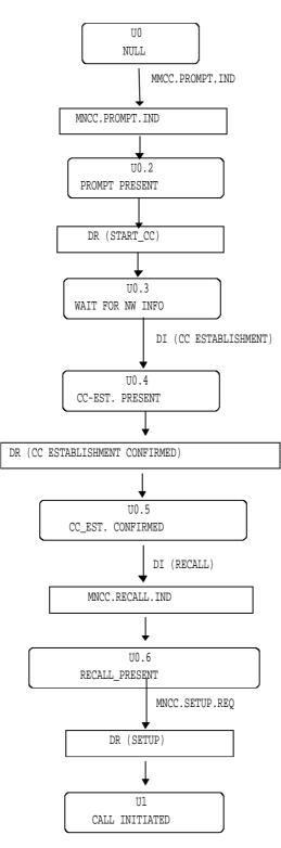
Figure5.1a.1/GSM 04.08: Overview call control protocol/MS side, extension:
