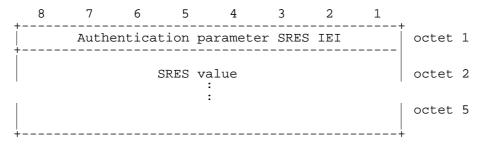
Figure 10.5.76/GSM 04.08: Authentication Parameter SRES information element
