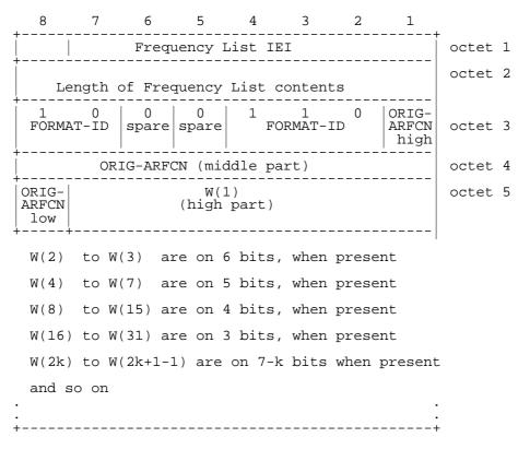
Figure 10.5.39/GSM 04.08: Frequency List information element (Range 128 format)
