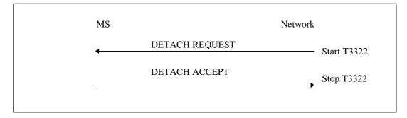
Figure 4.7.4/2 GSM 04.08: Network initiated GPRS detach procedure
