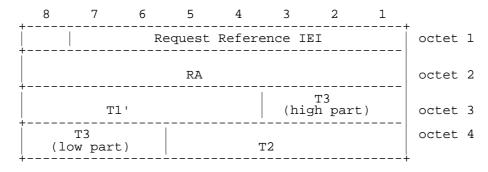
Figure 10.5.61/GSM 04.08: Request Reference information element
