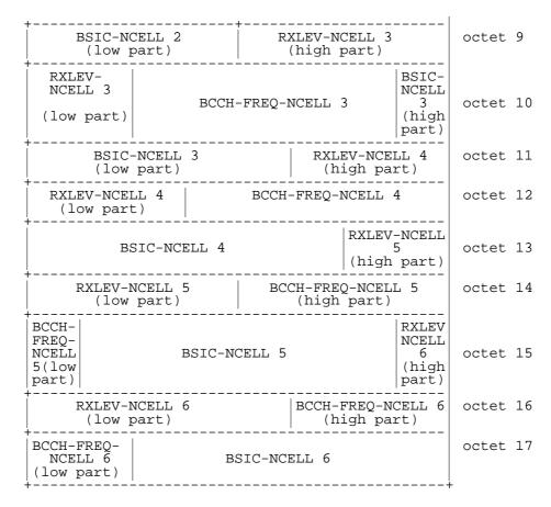
Figure 10.5.47/GSM 04.08: Measurement Results information element (continued)
