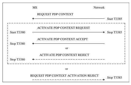
Figure 6.4/GSM 04.08: Network initiated PDP context activation procedure
