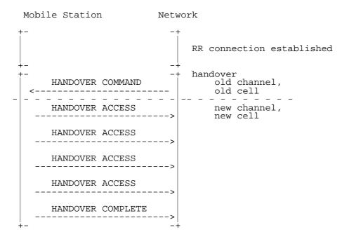
Figure 7.14/GSM 04.08: Handover to a finely synchronized cell, successful case
