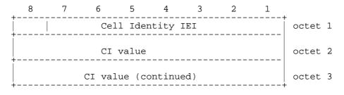
Figure 10.5.1/GSM 04.08: Cell Identity information element
