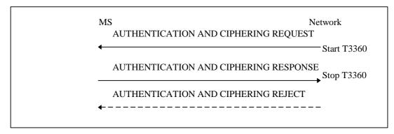
Figure 4.7.7/1 GSM 04.08: Authentication and ciphering procedure
