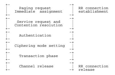
Figure 7.1/GSM 04.08: Components of structured procedures
