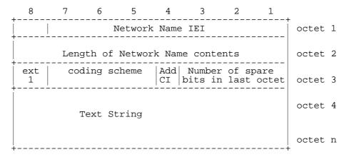
Figure 10.5.80/GSM 04.08: Network Name information element
