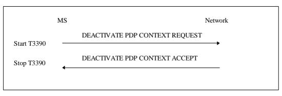
Figure 6.6/GSM 04.08: MS initiated PDP context deactivation procedure
