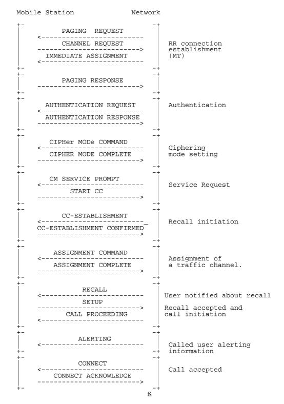
Figure 7.19/GSM 04.08: Network initiated mobile originating call establishment with assignment before A party alerting
