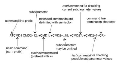
Figure 2: Basic structure of a command line
