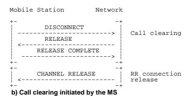
Figure 7.12/GSM 04.08 Call clearing
