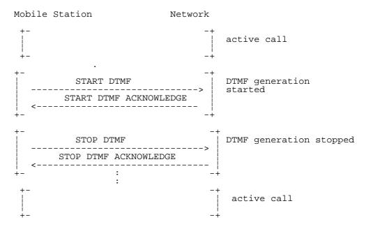
Figure 7.13/GSM 04.08 DTMF protocol control
