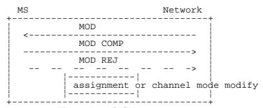
Figure 5.10b/GSM 04.08 In-call modification sequence initiated by network
