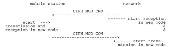
Figure 3.3/GSM 04.08 Ciphering mode setting sequence
