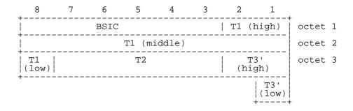
FIGURE 9.3/GSM 04.08 Frame synchronization information element
