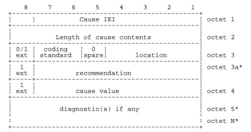
FIGURE 10.77/GSM 04.08 Cause information element
