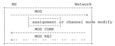
Figure 5.10a/GSM 04.08 In-call modification sequence initiated by MS
