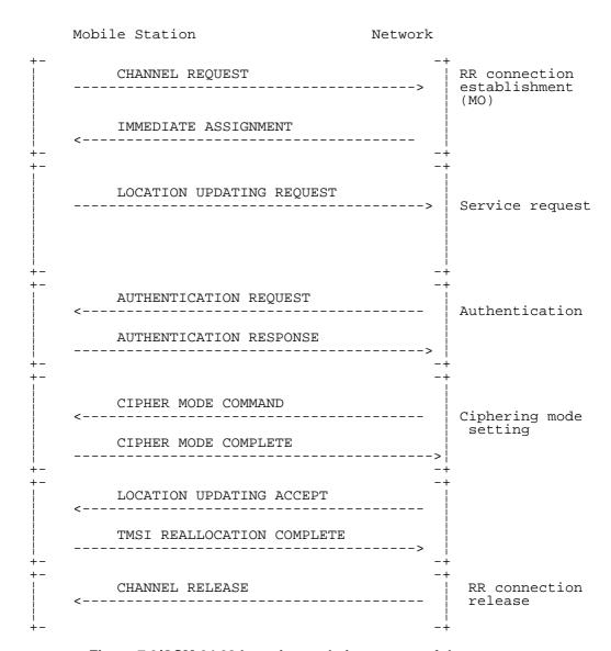
Figure 7.9/GSM 04.08 Location updating: successful case
