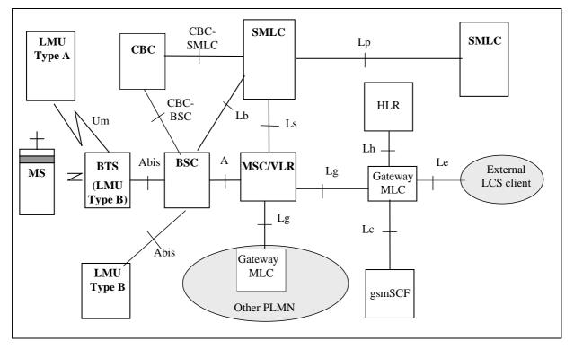
Figure 4: Configuration of a PLMN supporting LCS
