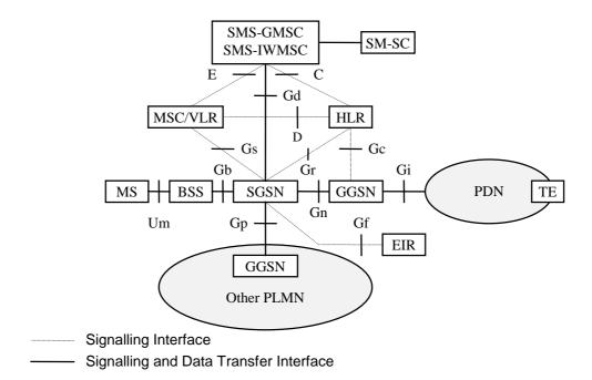
Figure 2: Configuration of a PLMN supporting GPRS
