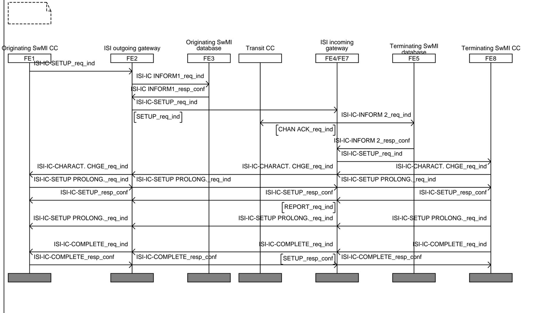
NOTE: The ISI-IC-SETUP PROLONGATION and -CHARACTERISTIC CHANGE request/indication information flows shown on the figure are optional.
