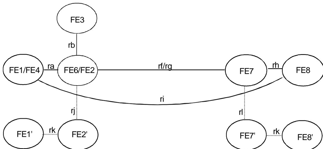
NOTE: Even though it is not a functional entity of ANF-ISIIC in this case (see subclause 5.1.2.4), FE4 has been shown in figure 4 to avoid showing a direct relationship between FE1 and FE6.
