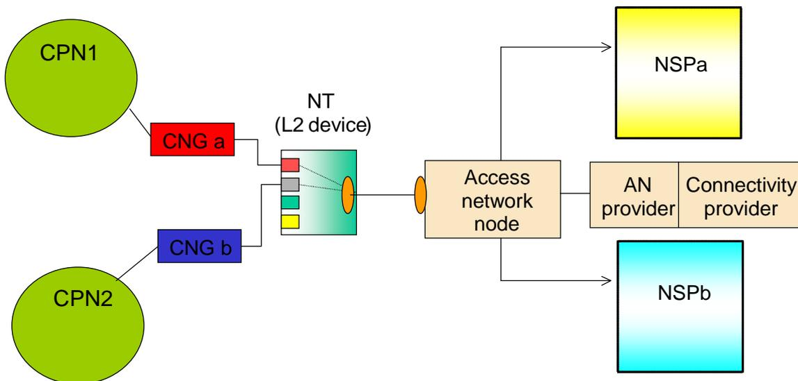
**Figure 4: Customer network architecture for multiple gateways, multiple service providers**
