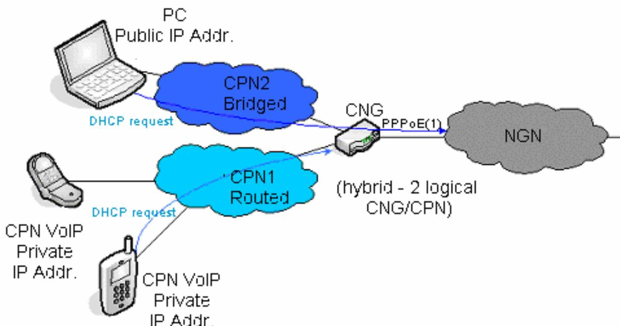
**Figure 2: Hybrid model with separate physical networks**
