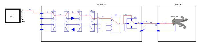
Figure B.2.1.4-3: Block Diagram of an EIRP/EIS test case with components from the gNB to the antenna (only portion of switch unit shown)
