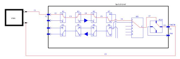
Figure B.2.1.4-4: Block Diagram of the calibration stage
