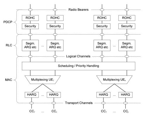
Figure 5.2.1-1: Layer 2 Structure for the DL
