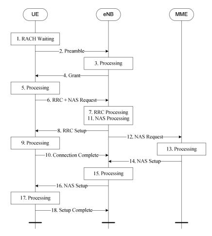
Figure 16.2.1-1: From Idle to Connected mode
