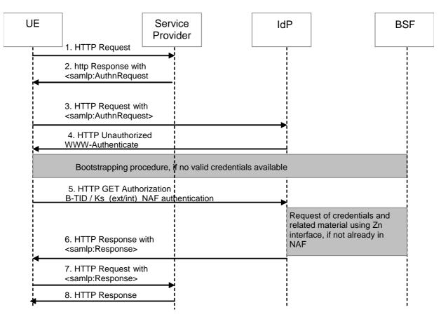
Figure 4.3-4: Message flow for SSO with <samlp:Response> and TLS with GBA
