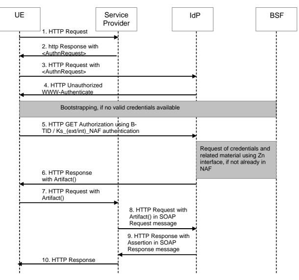
Figure 4.3-2: Message flow for SSO with Artefact transfer and usage of GBA
