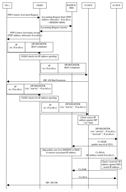
Figure 3: Message sequence for early IMS security showing interworking case where UE supports both fully compliant IMS and early IMS access security and network supports early IMS security only
