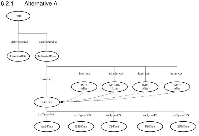
Figure 6.2.1-1: DIT Structure for UDC with alternative A
