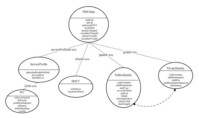
Figure 11.2.1-1: DIT Structure for IMS-Data with Alternative A
