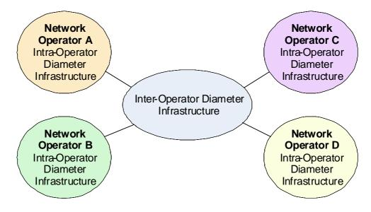
Figure A.1.1: High-level Diameter Infrastructure
