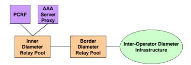
Figure A.2.1: Example of PCRF and AAA Server/Proxy connecting to inter-operator Diameter roaming infrastructure
