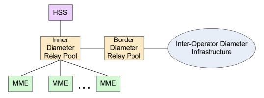
Figure A.1.2: Example Intra-Operator Diameter Infrastructure and its connectivity to inter-operator
