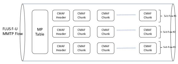
Figure 4: Structure of an MMTP flow as a FLUS F-U
