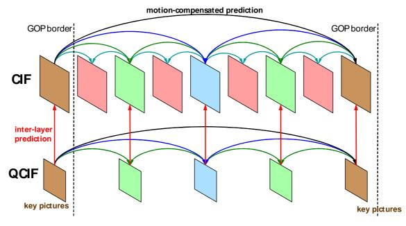
Figure 2: Example Prediction Structure for Spatial Scalability
