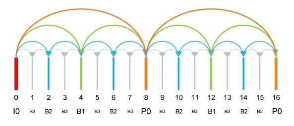
Figure 1: Temporal Scalability with Hierarchical B-Picture Structure in SVC
