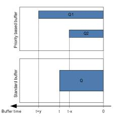
Figure 4: Priority (PBTS) buffer using different qualities (Q1 and Q2) vs. standard buffer with one quality (Q), with *t*+*y* respectively *t* being the maximum sustainable outage time
