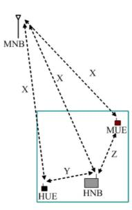
Figure 8.1-1: DL interference scenario
