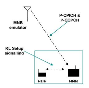
Figure 8.2-2: UL interference test setup
