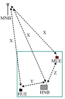
Figure 7.2.1.1-1: DL Interference Setup
