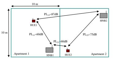
Figure 8.2.2.2-1: Inter-HNB uplink test set-up
