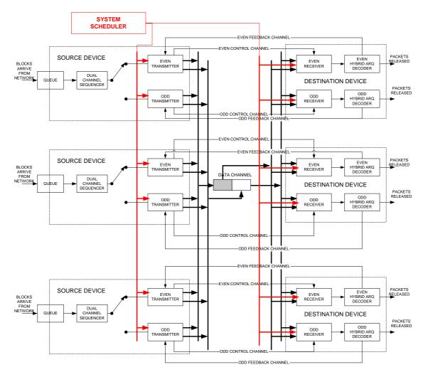
Figure 8: Multi-device/single data channel block diagram.
