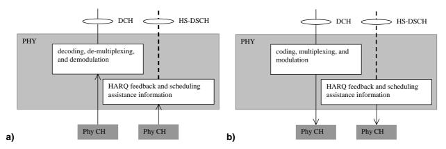
Figure 3: UL HS DSCH Physical Layer model, a) network side - b) UE side
