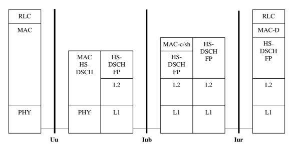
Figure 1: Radio Interface Protocol Architecture of HSDPA
