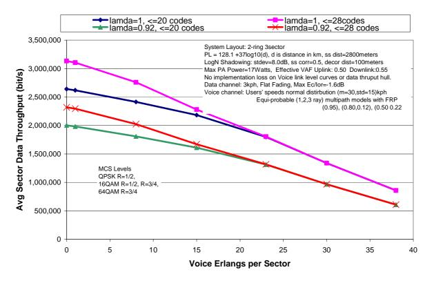
Figure 1: HSDPA Throughput vs. Voice Loading for different FRP (lamda) and for 20 and 28 OVSF codes where and Equal Average Power Scheduler is assumed.
