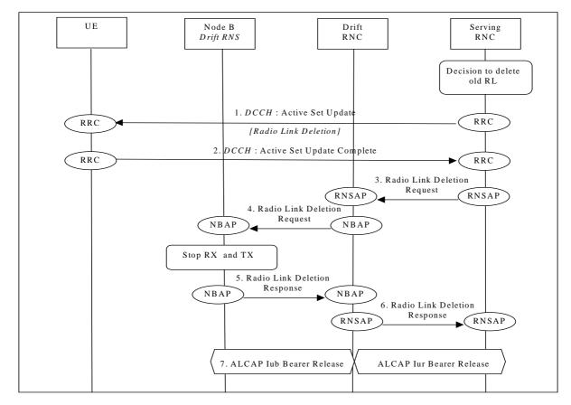
Figure 25: Soft Handover - Radio Link Deletion (Branch Deletion)
