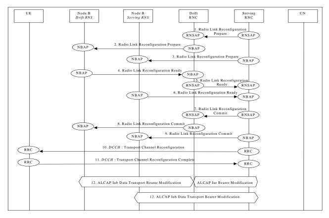
Figure 41b: Synchronised Transport Channel Reconfiguration, Bandwidth Decrease
