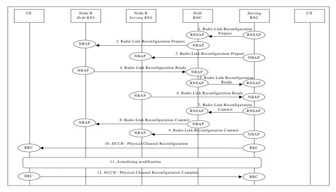
Figure 22: Physical Channel Reconfiguration (DCH)
