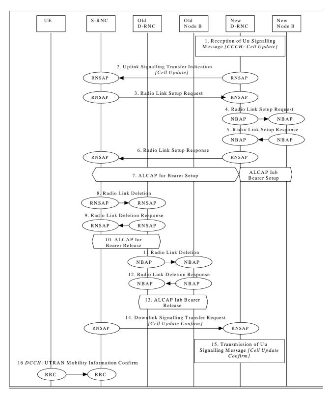
Figure 11: RRC connection Re-establishment (Anchor approach) - DCH Re-establishment
