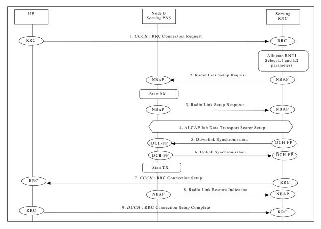
Figure 8: RRC Connection Establishment - DCH Establishment
