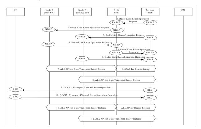
Figure 42: Unsynchronised Transport Channel Reconfiguration
