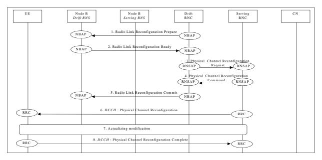
Figure 23: Physical Channel Reconfiguration (CRNC Controlled)
