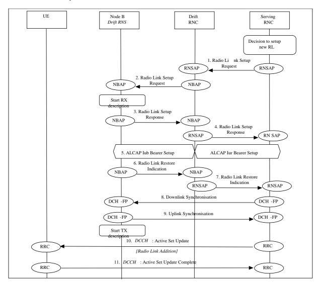
Figure 24: Soft Handover - Radio Link Addition (Branch Addition)
