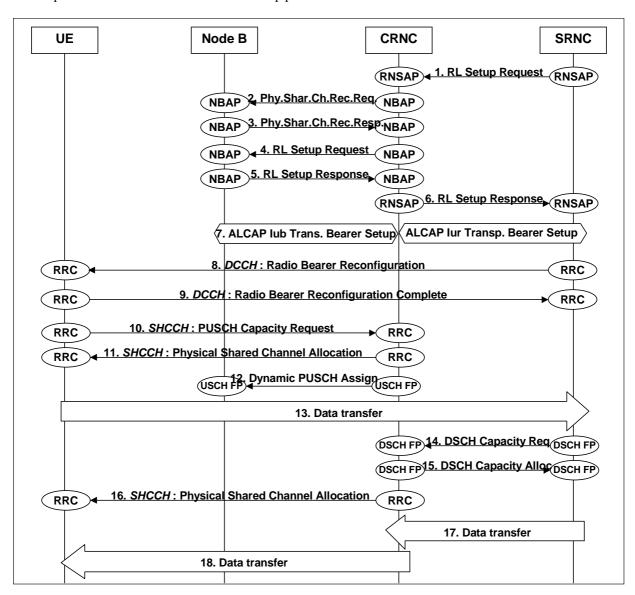
Figure 45a USCH/DSCH Configuration and Capacity Allocation
