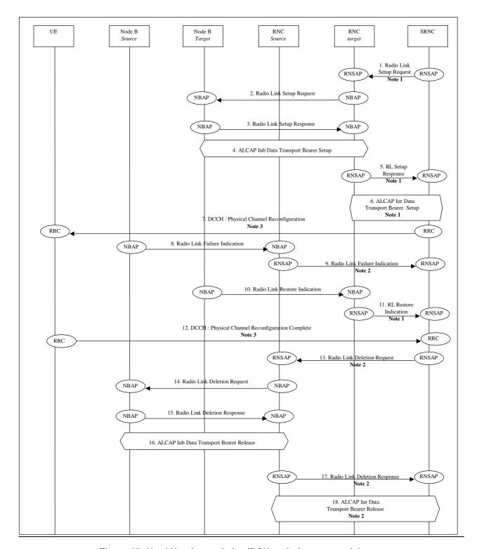
Figure 27: Hard Handover via lur (DCH on lur) - successful case
