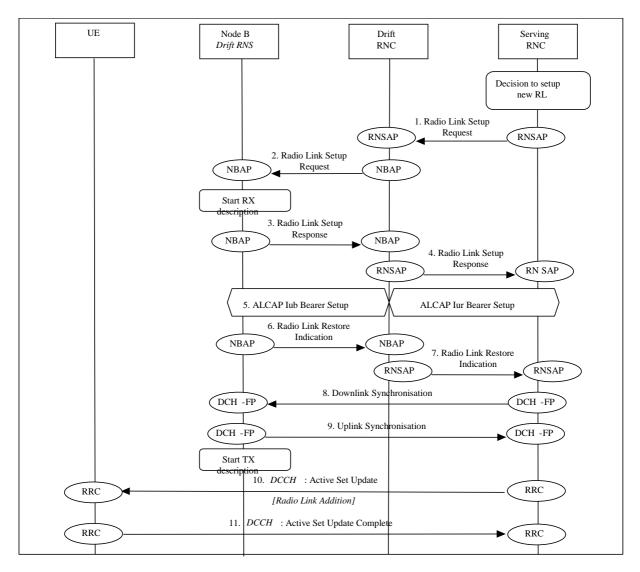
Figure 53: Soft Handover - Radio Link Addition (Branch Addition)
