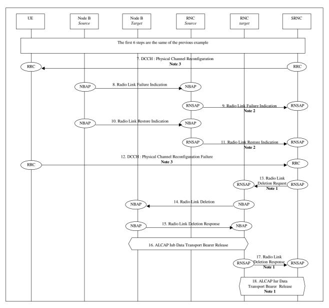
Figure 28: Hard Handover via lur (DCH on lur) - unsuccessful case.
