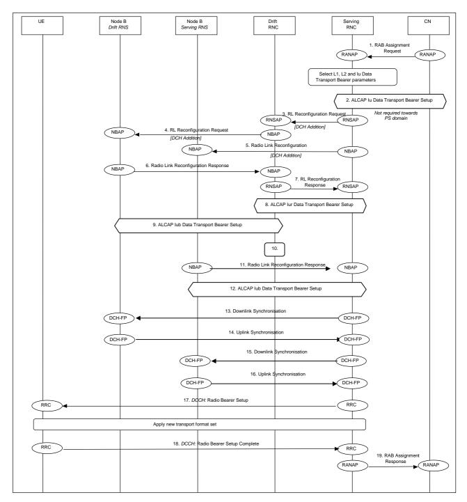
Figure 14: Radio Access Bearer Establishment - DCH - DCH Establishment - Unsynchronised
