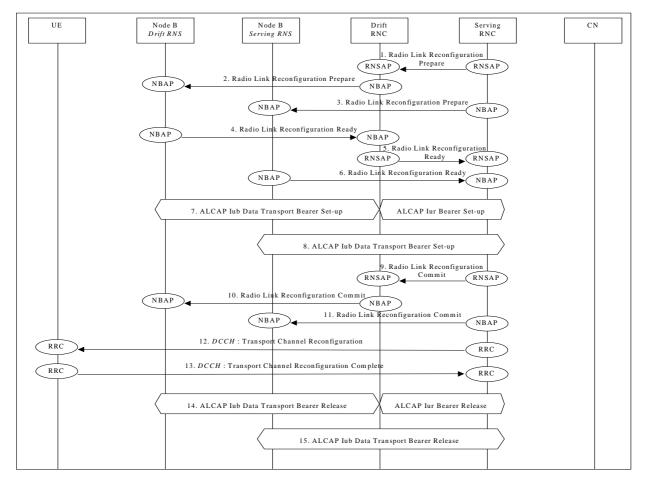
Figure 41: Synchronised Transport Channel Reconfiguration
