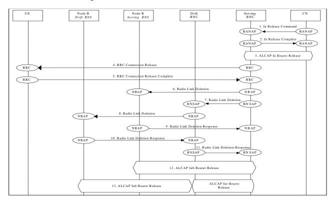
Figure 9: RRC Connection release of a dedicated channel
