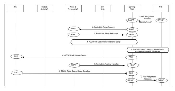
Figure 15: Radio Access Bearer Establishment – RACH/FACH - DCH Establishment – Unsynchronised
