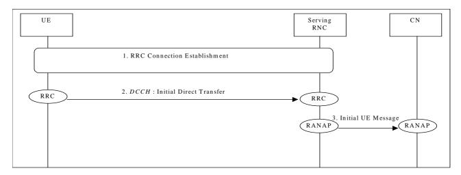
Figure 7: NAS Signalling Connection Establishment
