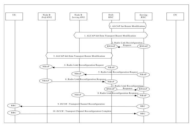
Figure 42a: Unsynchronised Transport Channel Reconfiguration, Bandwidth Increase
