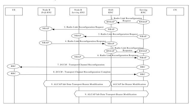
Figure 42b: Unsynchronised Transport Channel Reconfiguration, Bandwidth Decrease
