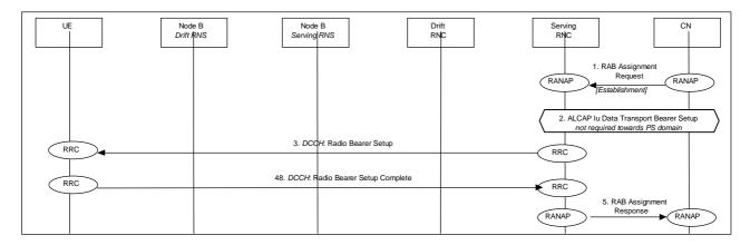
Figure 16: Radio Access Bearer Establishment – RACH/FACH – RACH/FACH Establishment – Unsynchronised
