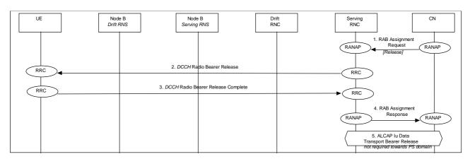
Figure 19: Radio Access Bearer Release - RACH/FACH - RACH/FACH Release
