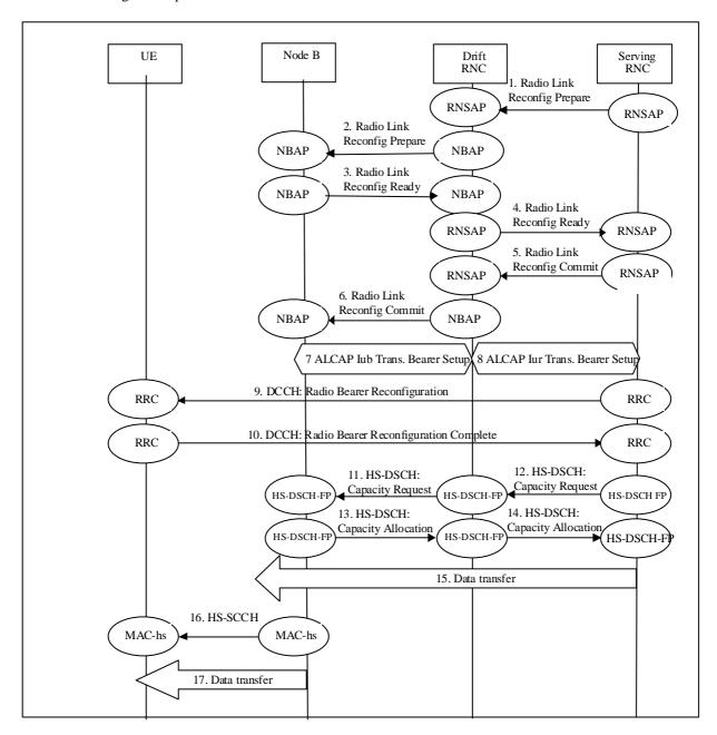
Figure 45b: HS-DSCH Configuration and Capacity Allocation
