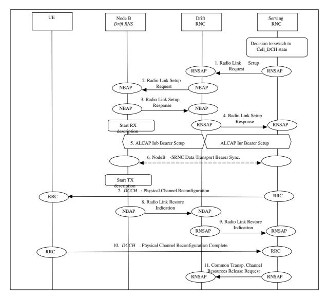
Figure 45b Switching from Cell\_FACH to Cell\_DCH State via lur
