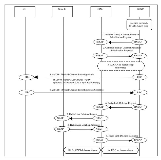
Figure 45c Switching from Cell\_DCH to Cell\_FACH State via lur
