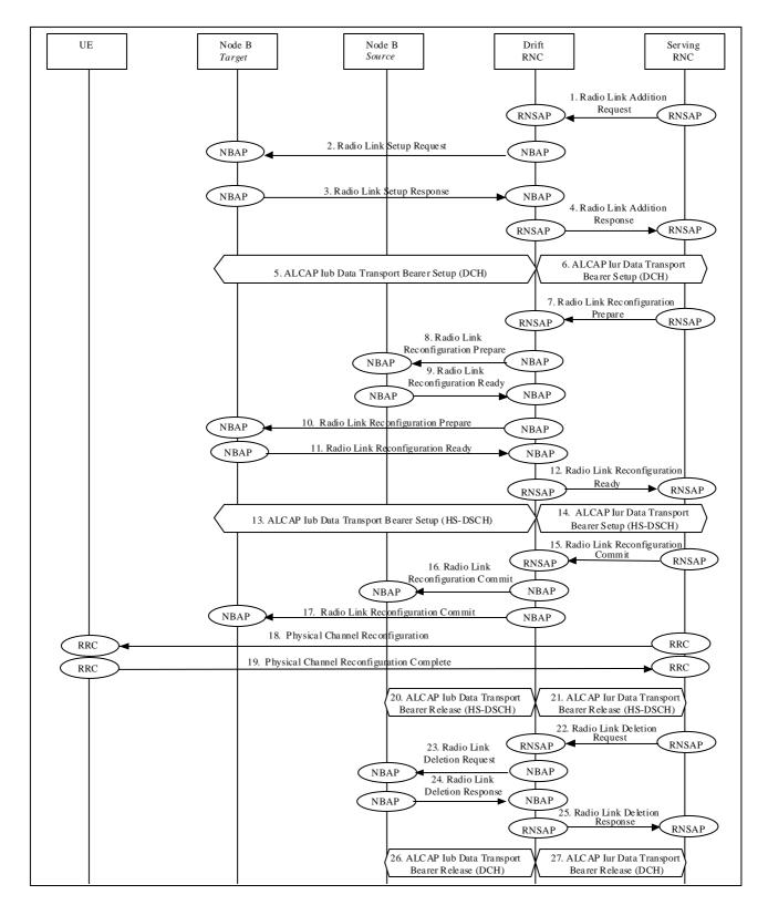
Figure 29a: Inter-Node B (intra DRNC) synchronised serving HS-DSCH cell change at hard handover
