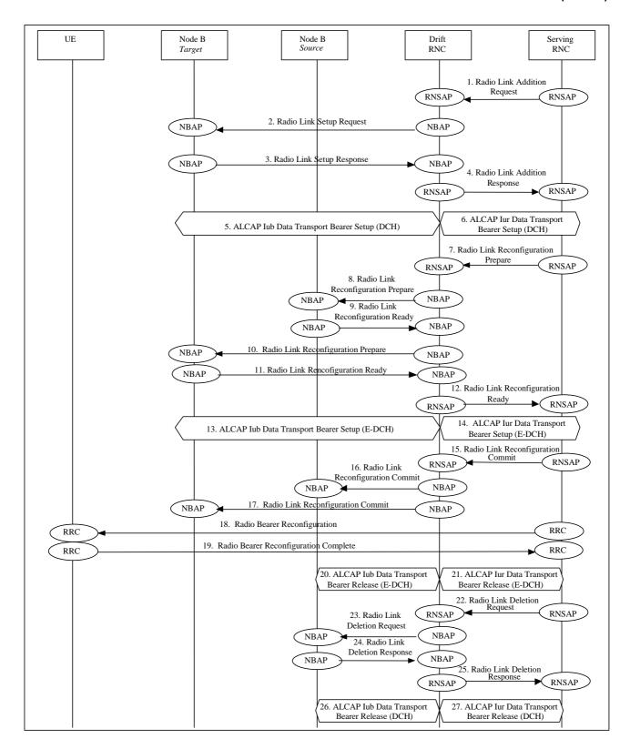
Figure 56: Inter-Node B (intra DRNC) synchronised serving E-DCH cell change at hard handover
