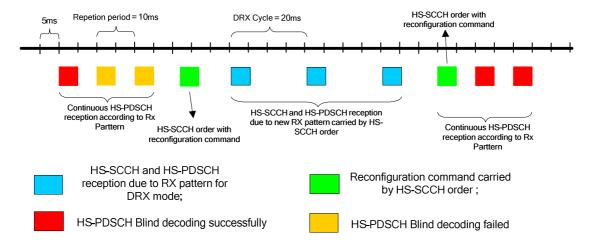
1) When NodeB detect the state switch from active to silent according to the buffer of UE, NodeB shall send reconfiguration command by HS-SCCH order to reconfigure the physical resource of UE. The physical resource include the channel code resource and Rx pattern
