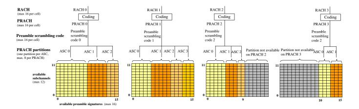
Figure H.1: Examples of FDD RACH/PRACH configurations in a cell
