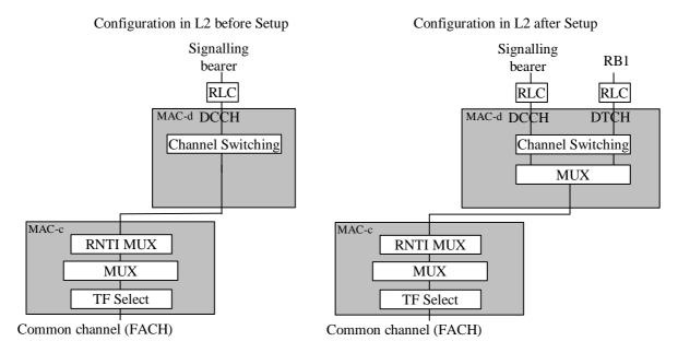
Figure 7-1: Configuration of L2 in the UTRAN DL before and after the RB setup
