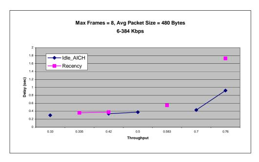
Figure G-1: Delay vs. Throughput
