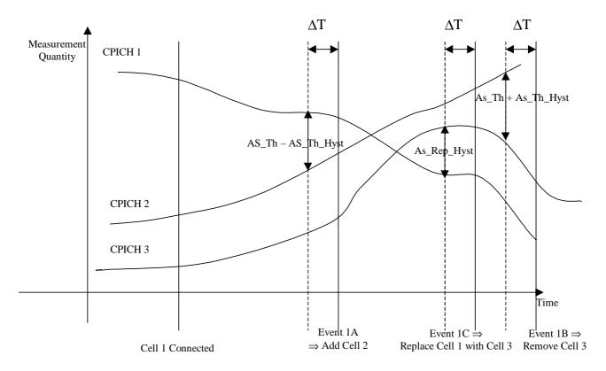
Figure 5-1: Example of Soft Handover Algorithm
