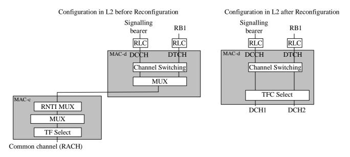
Figure 7-2: Configuration in the UTRAN UL before and after the Physical channel reconfiguration
