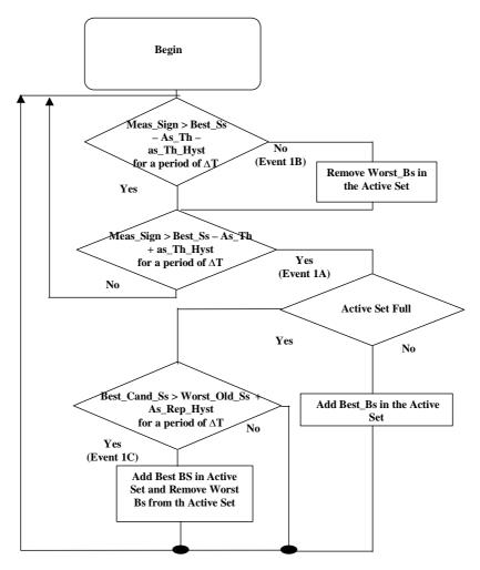
Figure C-1: flow-chart of a Soft Handover algorithm
