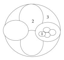
Figure 4-1: Example of Hierarchical Cell Structure
