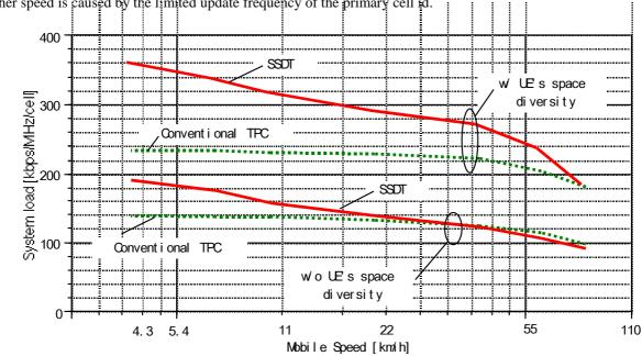
Figure D-1: Capacity versus Doppler frequency for SSDT and conventional TPC (normal SHO)
