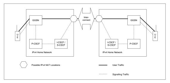
Figure A.2-2: Non-roaming IPv4 IM CN subsystem with IPv4 IM CN subsystem
