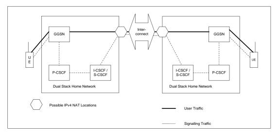
Figure A.2-4: Non-roaming Dual Stack IM CN subsystem with Dual Stack IM CN subsystem
