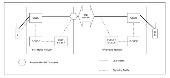
Figure A.2-1: Non-roaming IPv4 IM CN subsystem with IPv6 IM CN subsystem
