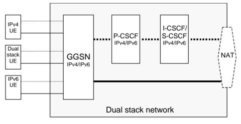
Figure 5-3: Non-roaming dual Stack IM CN subsystem
