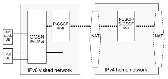
Figure A.1-3: IMS roaming access - IPv6 visited network, IPv4 home network
