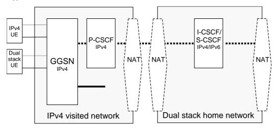
Figure A.1-4: IMS roaming access - IPv4 visited network, dual stack home network
