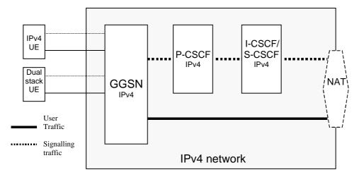
Figure 5-2: Non-roaming IPv4 IM CN subsystem
