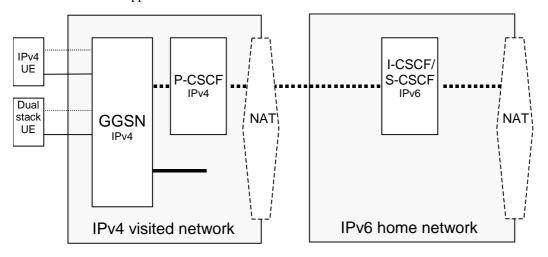
Figure A.1-2: IMS roaming access – IPv4 visited network, IPv6 home network
