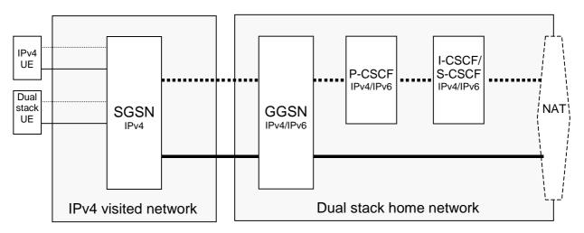
Figure 5-6: GPRS roaming – IPv4 visited network, dual stack home network
