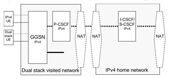
Figure A.1-1: IMS roaming access – IPv4 visited network, IPv4 home network
