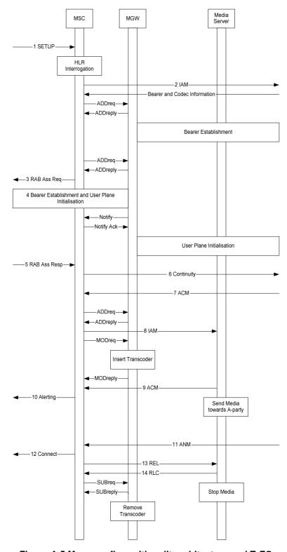
Figure A.5 Message flow with split architecture and TrFO
