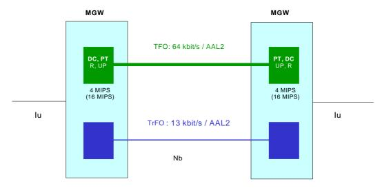
Figure 5.1.4-2: Bandwidth and resource usage for RNC to RNC call via BICN
