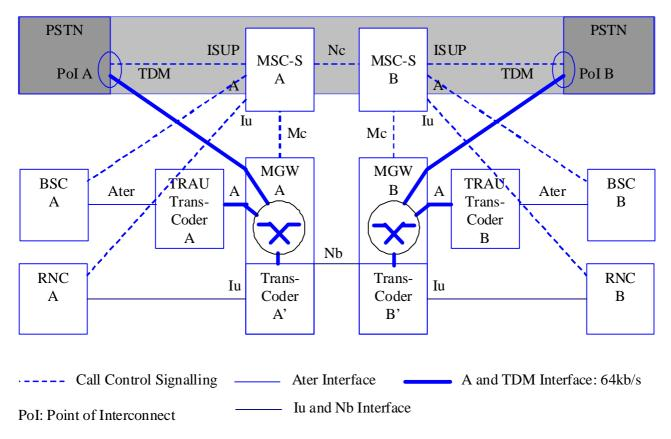
Figure 4.3-1: Bearer Independent Core Network with A- and lu-interfaces from Release 4 onwards
