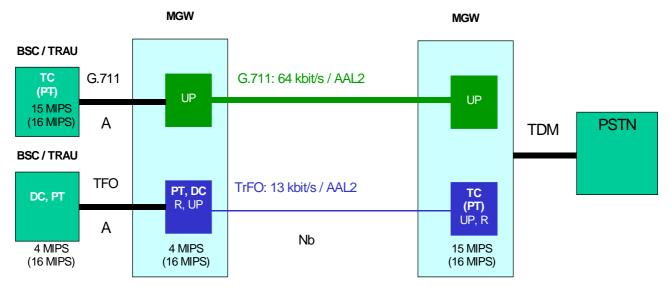
NOTE: The MIPS values in brackets() indicate the DSP-resource usage in the short TFO-setup phase, when TC is used.
