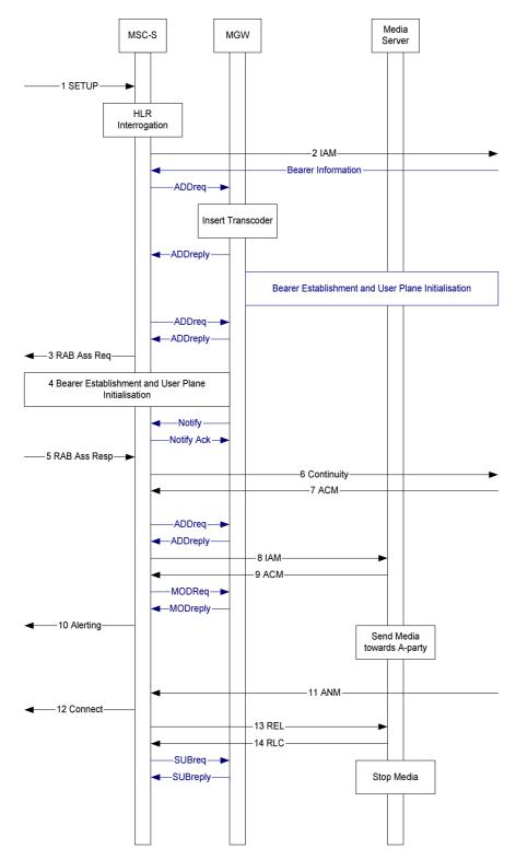
Figure A.4: Message flow with split architecture without TrFO
