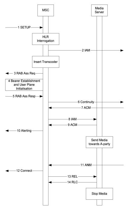
Figure A.2: Message flow in a R99 network
