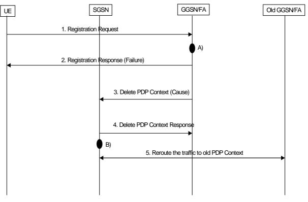
Figure 10.2a: Mobile IP registration failure
