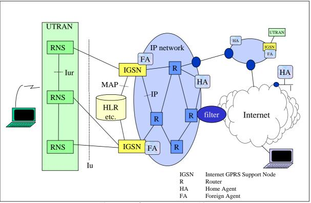
Figure 11a: Step 3 network architecture
