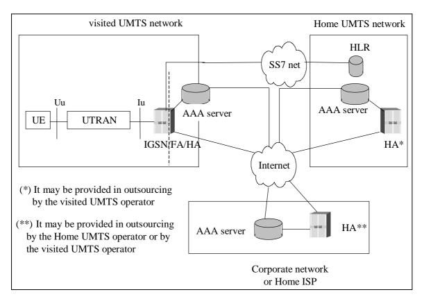
Figure 8.7.1a: UE attached to the Home UMTS operator
