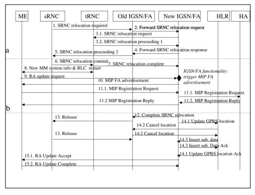
Figure 11.6a: SRNS relocation in a step 3 network
