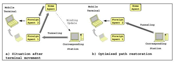
Figure A.4: Mobile terminal movement without notification to the previous foreign agent
