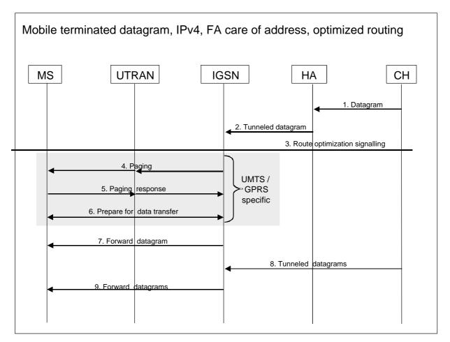
Figure 11.7.2b: Delivery of mobile terminated datagrams, optimised routing
