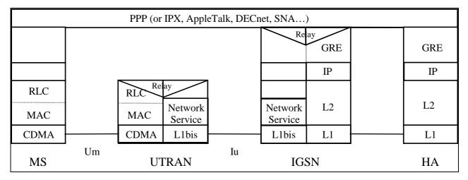
Figure 11.8.2a: Multiprotocol support in Mobile IP(+)
