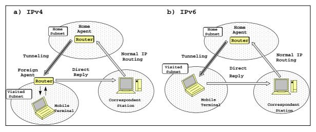
Figure A.1: Basic architecture for supporting IP mobility
