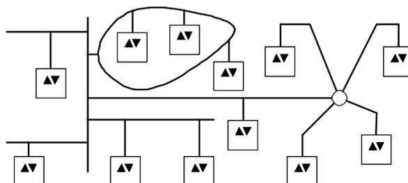
Figure 8: Combined topologies for HBES cabling and device connection
