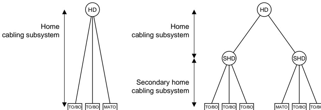
Figure 4: BCT/ICT cabling topologies of EN 50173-4 [i.4]
