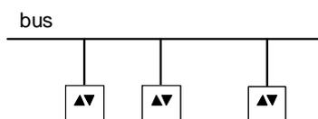
Figure 5: Bus topology for HBES cabling and device connection
