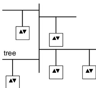
Figure 6: Tree topology for HBES cabling and device connection
