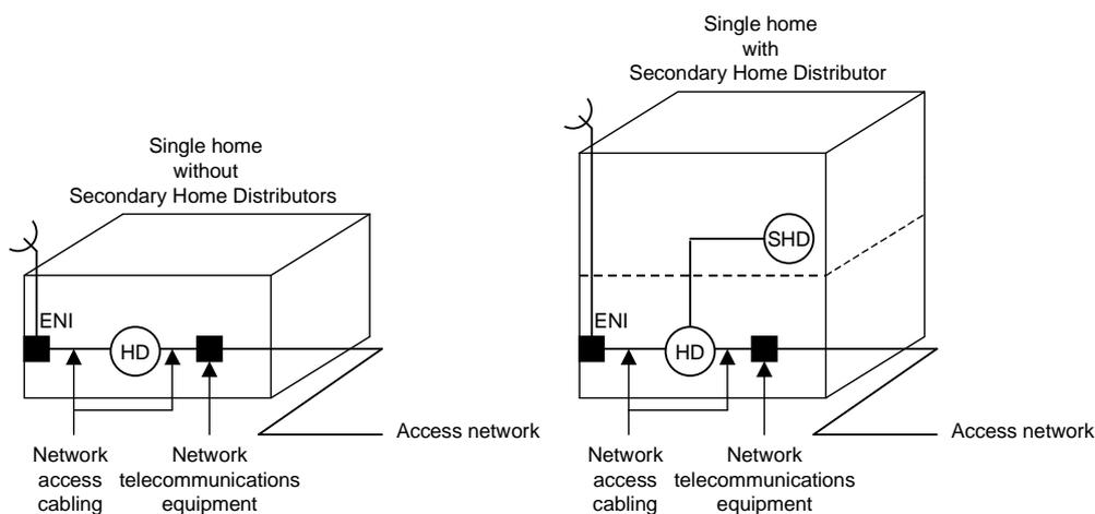
**Figure 2: Examples of generic cabling within the home according to EN 50173-4 [i.4]**
