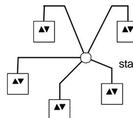
Figure 7: Star topology for HBES cabling and device connection
