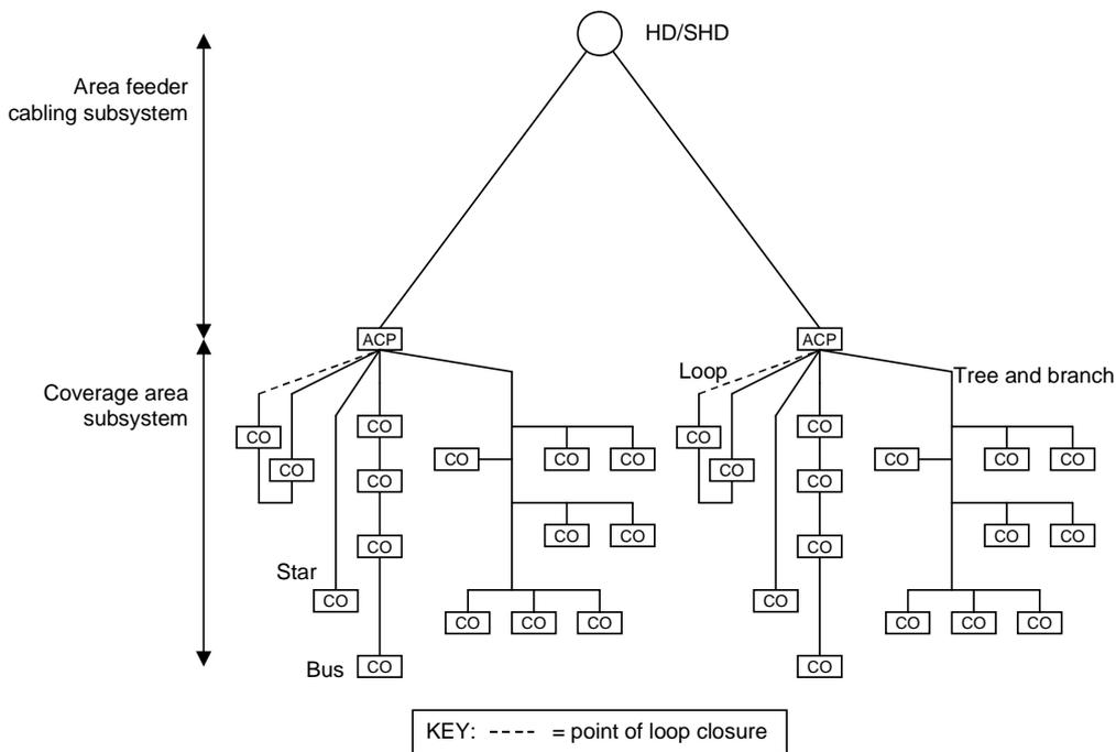
Figure 3: CCCB cabling topologies of EN 50173-4 [i.4]
