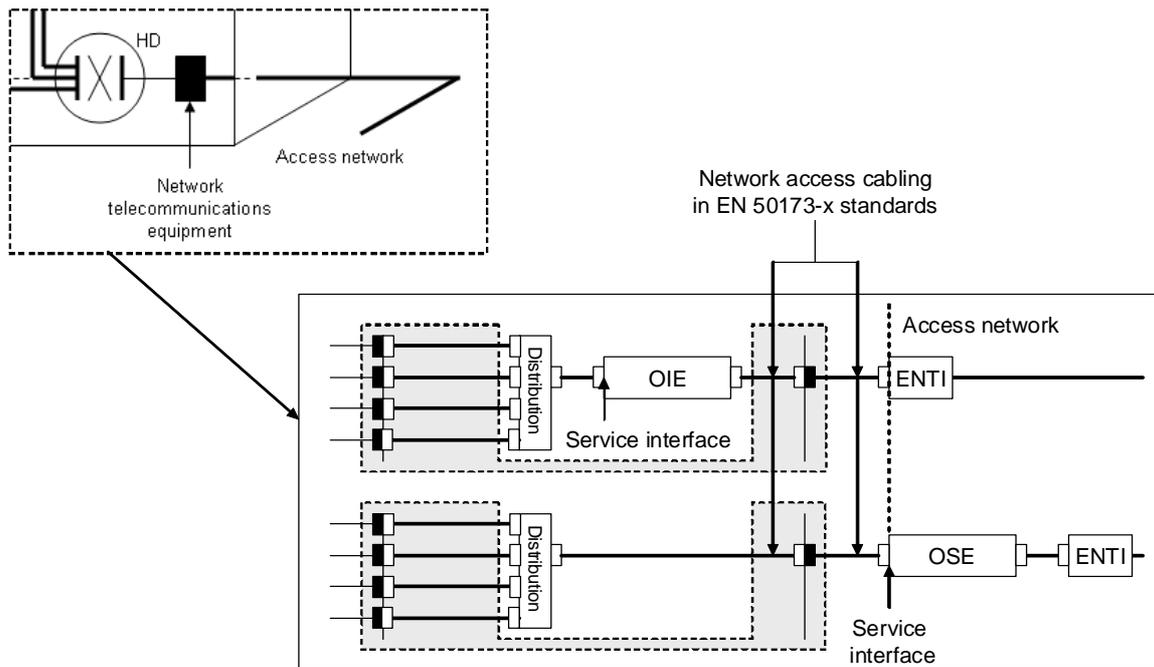
**Figure 9: Network access cabling and equipment**
