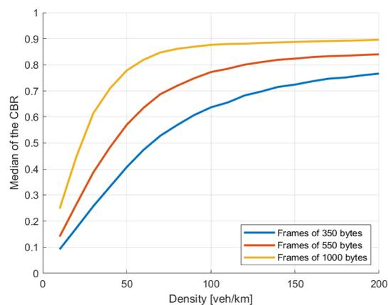
**Figure 2: Median of the CBR varying the density**
