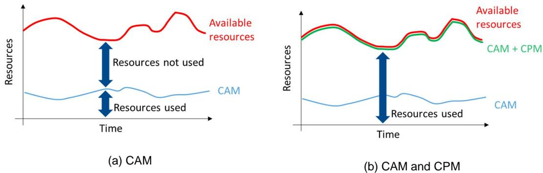
Figure 12: Illustration of resources consumed by CAM and CPM
