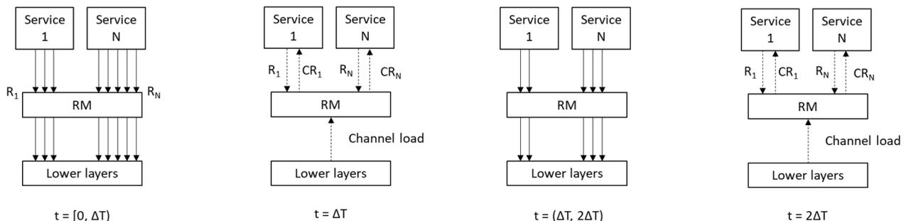
**Figure 18: Interaction between RM and services for bandwidth management**
