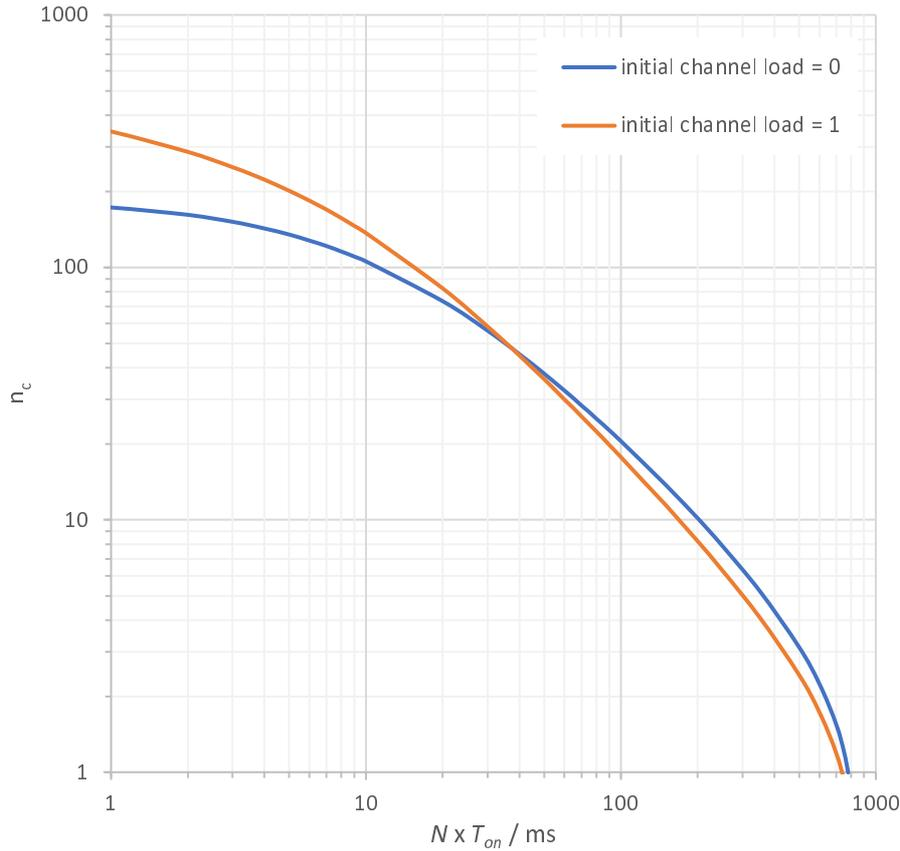
**Figure C.15: Number of time steps to reach  $\pm 5\%$  deviation from the equilibrium channel load when starting from different initial channel loads for the adaptive congestion control with parameter values given in Table 3 of ETSI TS 102 687 [i.14]**
