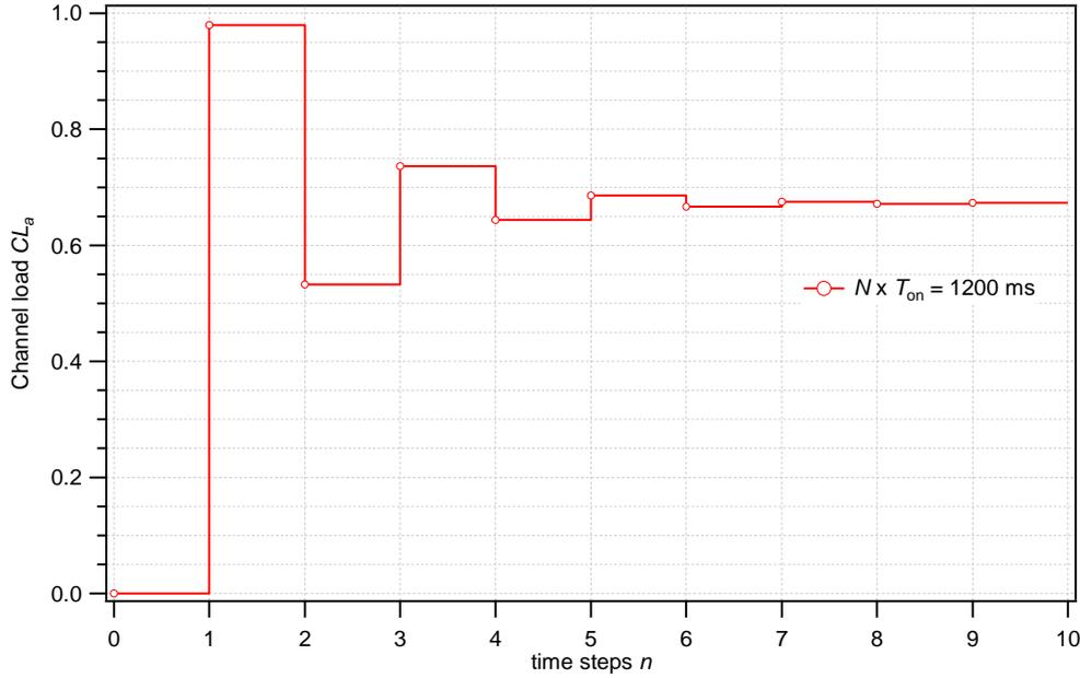
**Figure C.14: Channel load of adaptive congestion control for  $N \times T_{on} = 1\,200$  ms resulting from equation (C.53) for the parameter values given in Table 3 of ETSI TS 102 687 [i.14]**
