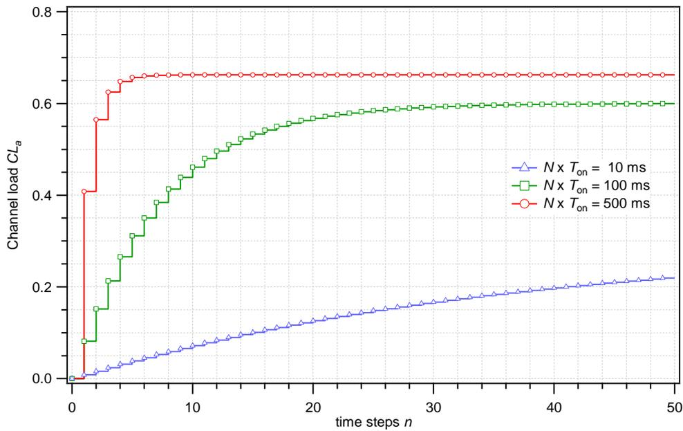
**Figure C.13: Channel load of adaptive congestion control for different values of  $N \times T_{on}$  resulting from equation (C.53) for the parameter values given in Table 3 of ETSI TS 102 687 [i.14]**
