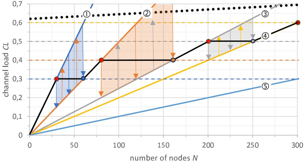
**Figure C.9:  $CL$  resulting from the  $T_{off}$  values taken from the reactive DCC**
