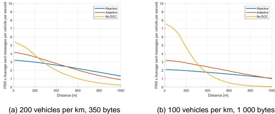
**Figure 7: Average number of messages per second correctly received from a station at a given distance**
