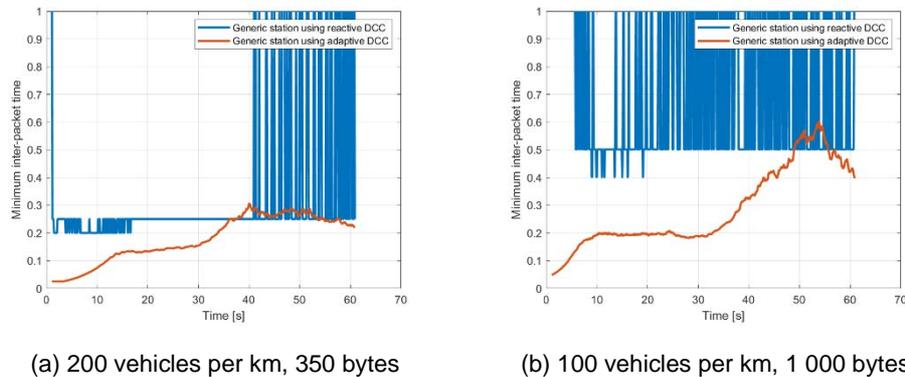
**Figure 8: Variation of the minimum inter-packet generation interval for randomly selected stations varying time**
