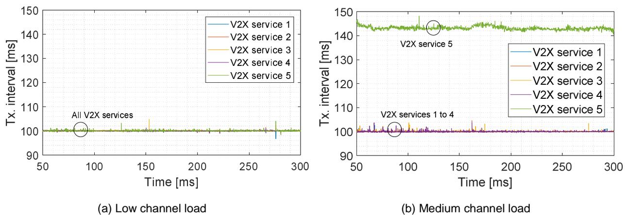
**Figure E.2: Time evolution of transmission interval of different services**
