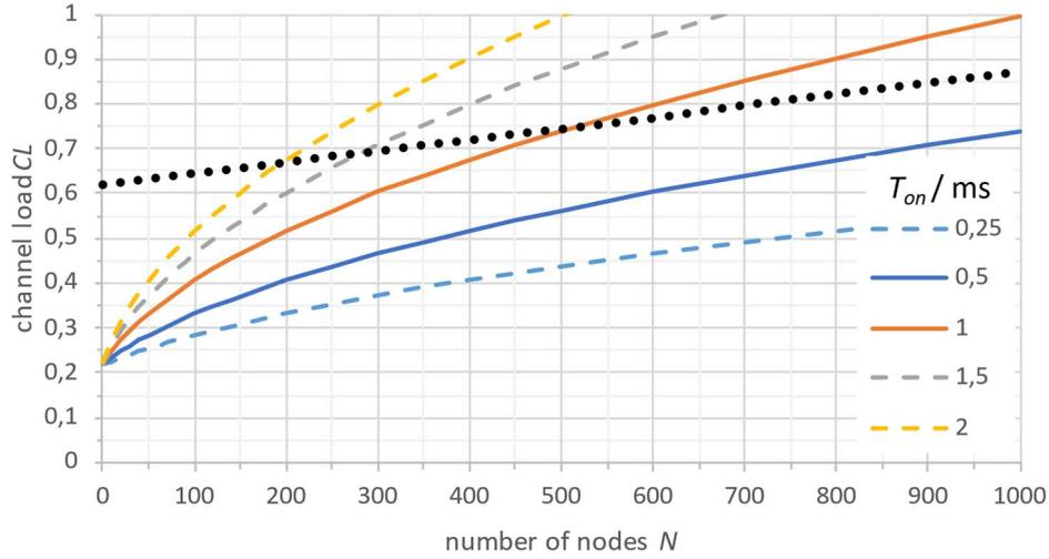
Figure C.3: Equilibrium channel load of reactive congestion control for  $T_a$  and  $T_b$  from Table C.1 for  $0,5 \text{ ms} < T_{on} \leq 1 \text{ ms}$
