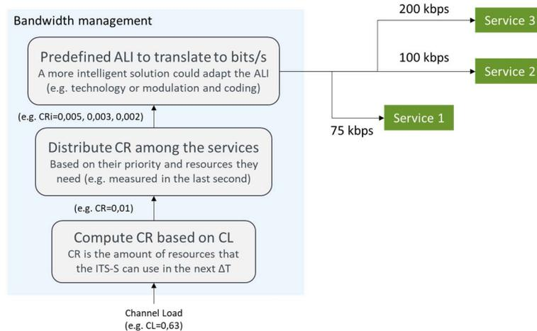
**Figure 17: Example of basic bandwidth management**
