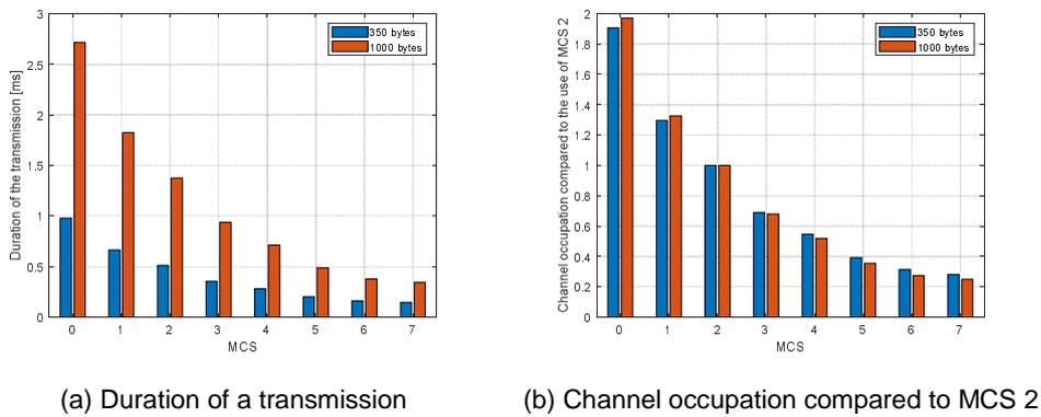
**Figure 9: Impact on channel occupation of data-rate control in ITS-G5**
