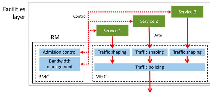
Figure 15: Architecture and mechanisms for Resource Management (RM) at Facilities layer
