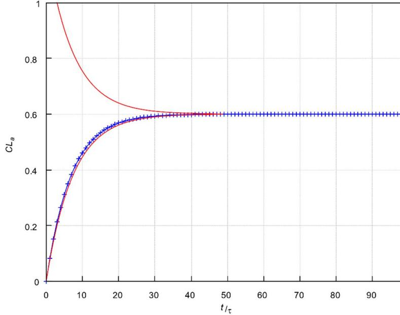
**Figure C.11: Analytic and numeric solution of the continuous time adaptive congestion control for  $N = 100$ ,  $T_{on} = 1$  ms, and the parameters given in in Table 3 of ETSI TS 102 687 [i.14]**
