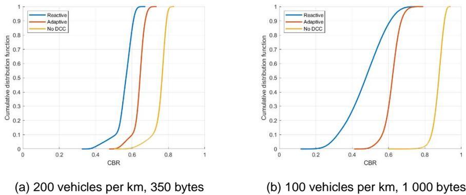
**Figure 6: Cumulative distribution function of the measured CBR**
