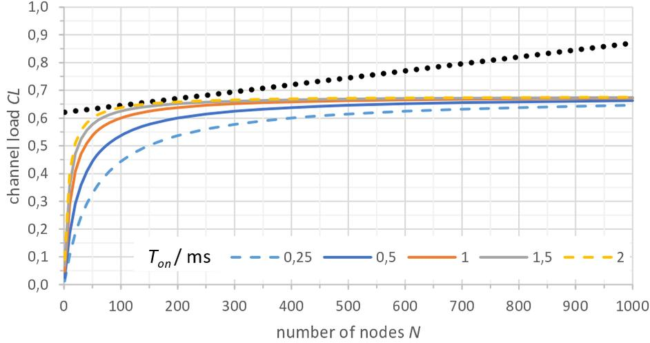
**Figure C.10: Equilibrium channel load of adaptive congestion control for the parameter values given in Table 3 of ETSI TS 102 687 [i.14]**
