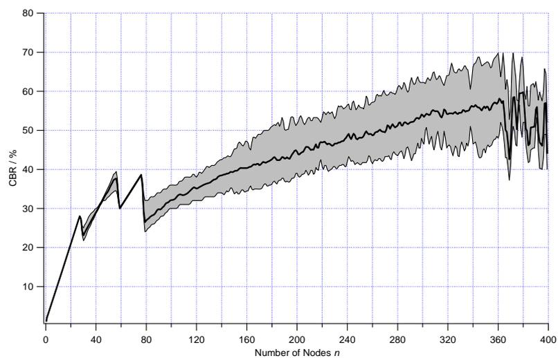
**Figure D.3: Bounded stability for a reactive DCC according to C2C-CC: "Vehicle C-ITS station profile #2037", RS\_BSP\_240 [i.34] for  $T_{on} = 1$  ms and 200 ms CBR measurement time**
