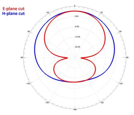
Figure 1: Typical Antenna Radiation Pattern
