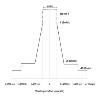
Figure A.2: Proposed Spectral Mask
