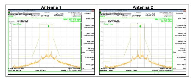
Figure B.1: Transmitter Spectrum Mask at 917,5 MHz
