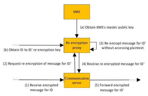
Figure 10: Proxy re-encryption using an IBE re-encryption scheme
