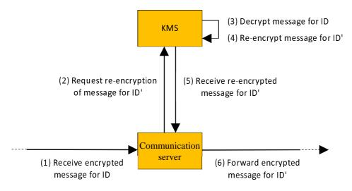
Figure 9: Proxy re-encryption using the KMS
