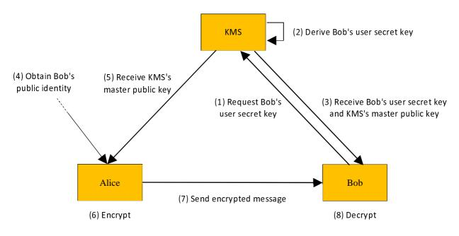
Figure 2: General model of IBE cryptosystems
