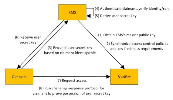
Figure 11: Model for resource access control using IBE
