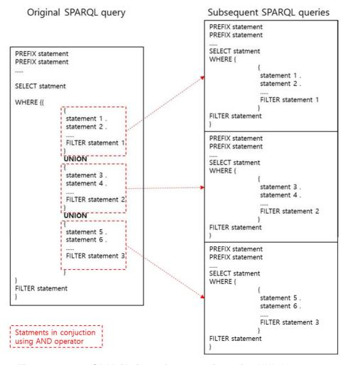
Figure 7.2.3.2-1: SPARQL Query fragmentation using UNION Operator
