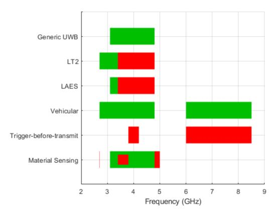
Figure 1: Duty cycle applicability in UWB regulations
