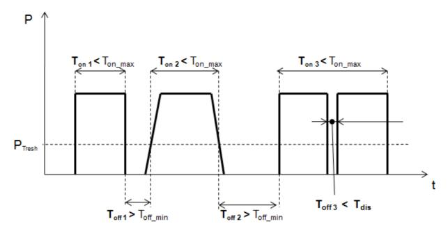
Figure 2: Illustration Pthresh, Ton, Toff and Tdis
