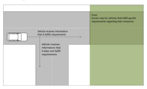
Figure 3: Illustration use-case access restriction based on vehicle type or vehicle emission type
