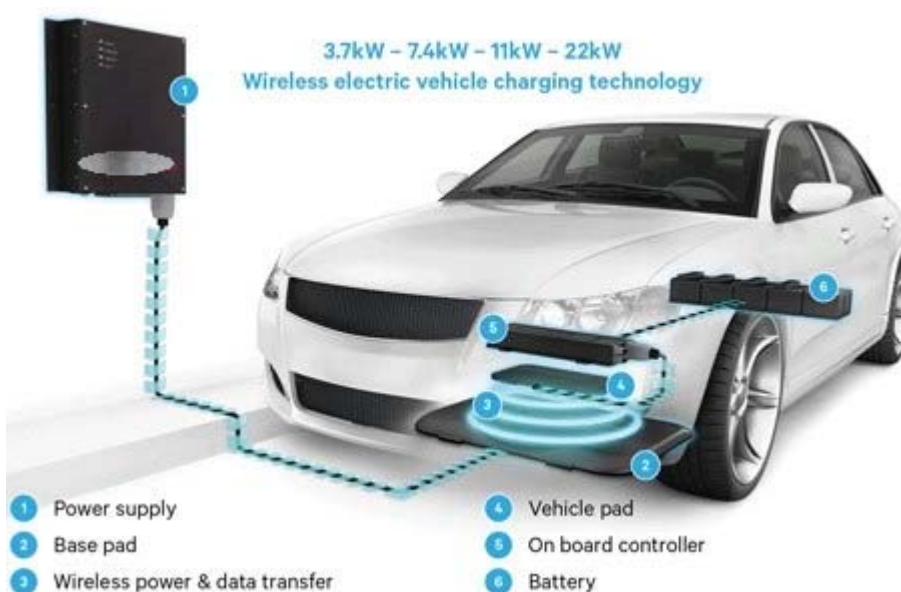
Figure 2: Schematical design of a typical WPT-EV system logo qualcomm
