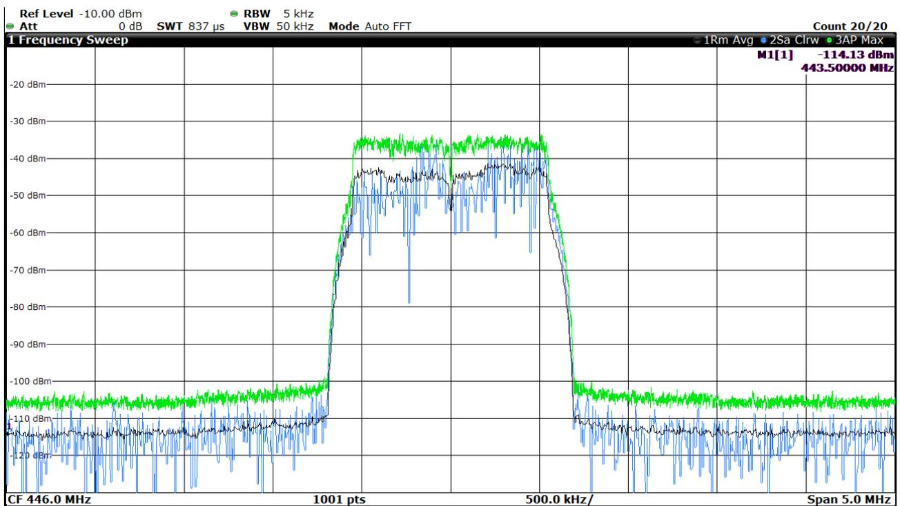
Figure H.12: 1,4 MHz LTE Signal E-TM3.3
