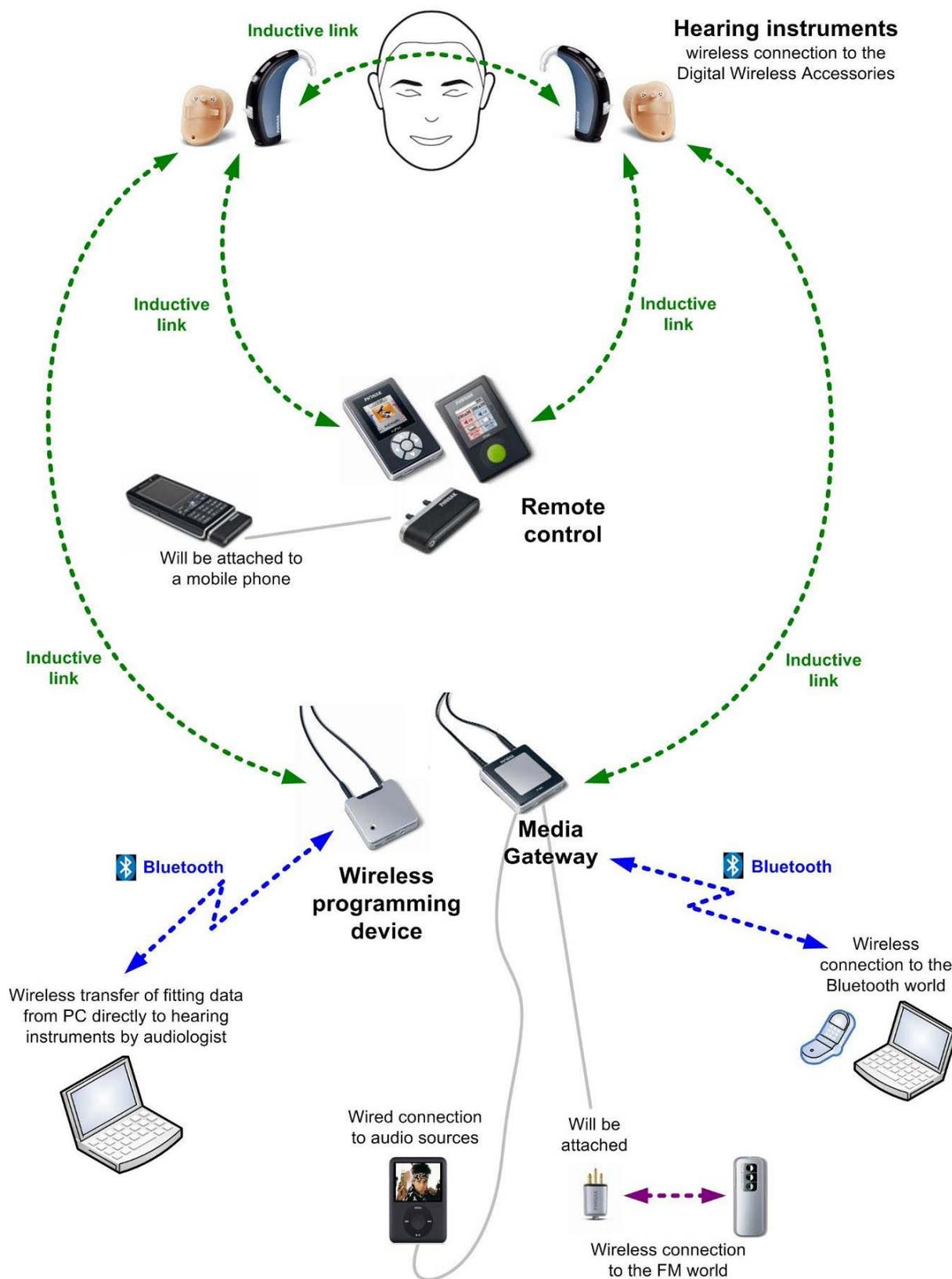
Figure I.3: Typical ALD system: the audio input can be from a human or the range of devices shown above
