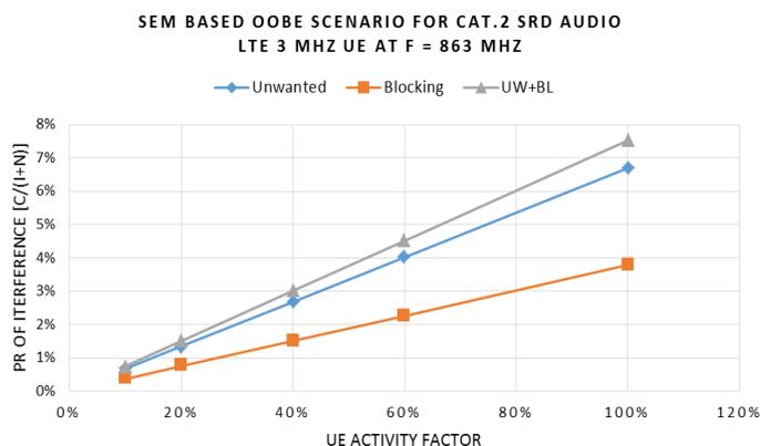
**Figure F.2: Probability of interference for Cat.2 SRD Audio**
