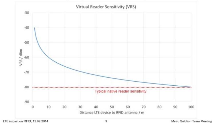
**Figure G.3: Loss in sensitivity loss of interrogator due to LTE OOB emissions**
