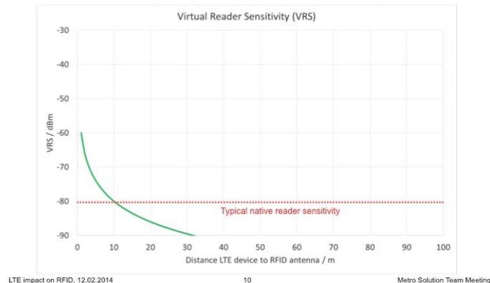
**Figure G.4: Improvement possible with a reduction in LTE OOB emissions**
