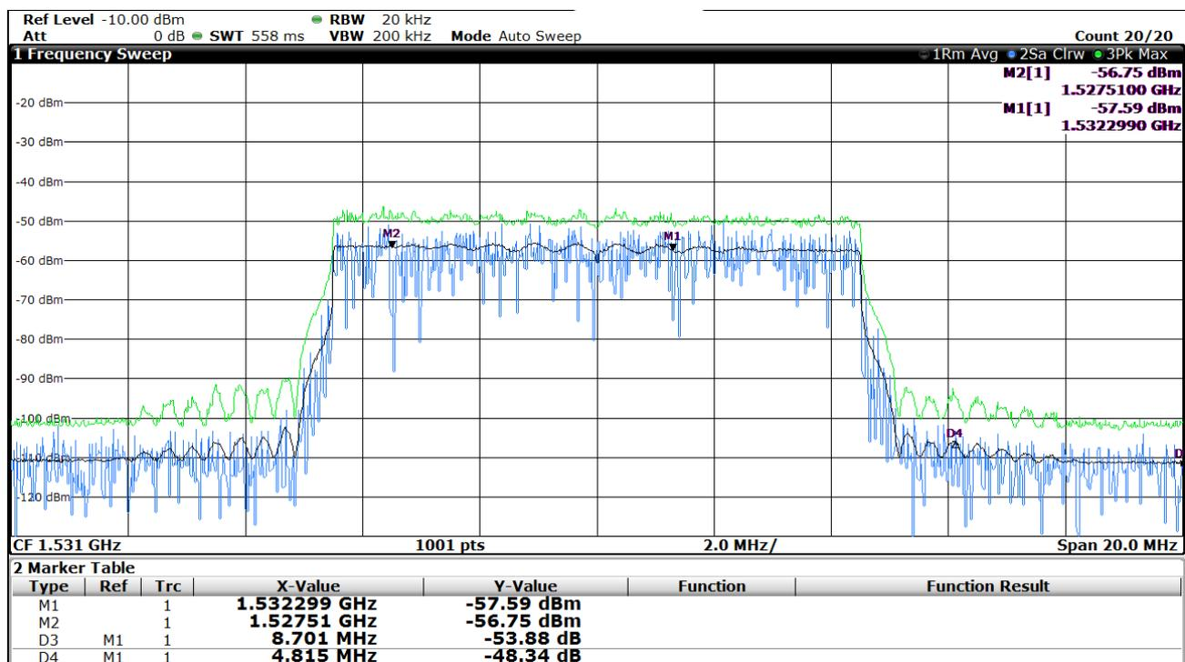
Figure H.1: E-TM1.1 signal, -33 dBm mean power
