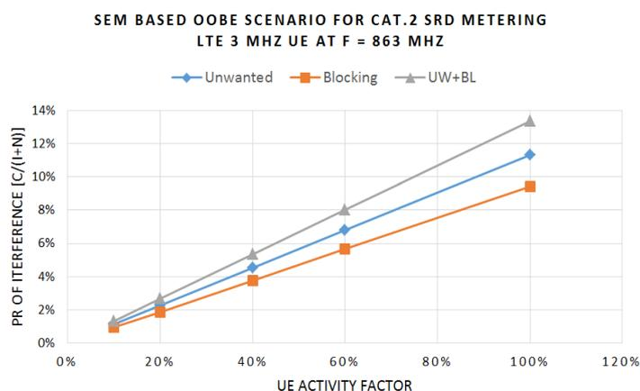
**Figure F.1: Probability of interference for Cat.2 SRD Metering**
