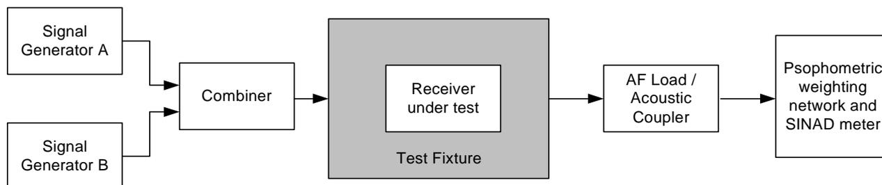
**Figure H.13: Measurement arrangement**
