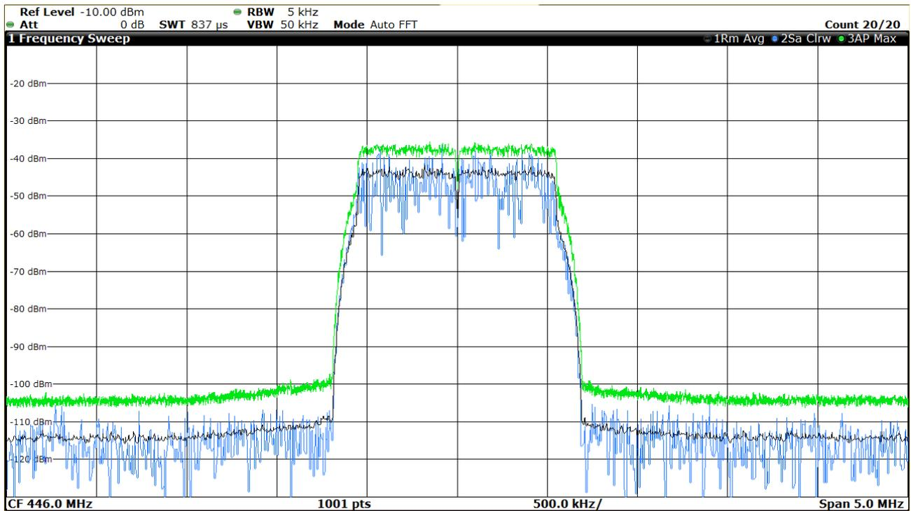
Figure H.7: 1,4 MHz LTE Signal E-TM1.1
