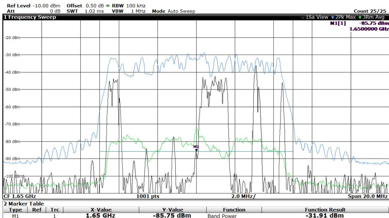
Figure H.4: E-TM2 signal ("idle mode"), fast sweep
