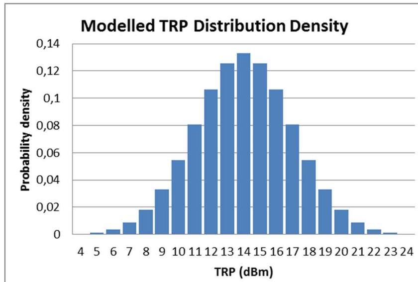
Figure F.5: Modelled TRP Distribution Density (HH)
