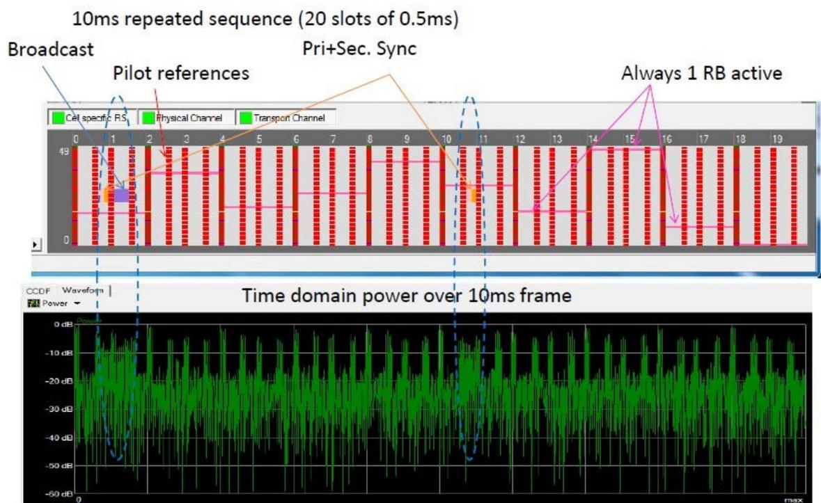
**Figure B.7: E-TM2 signal as generated by Agilent Signal Studio (Source: Sony Europe)**
