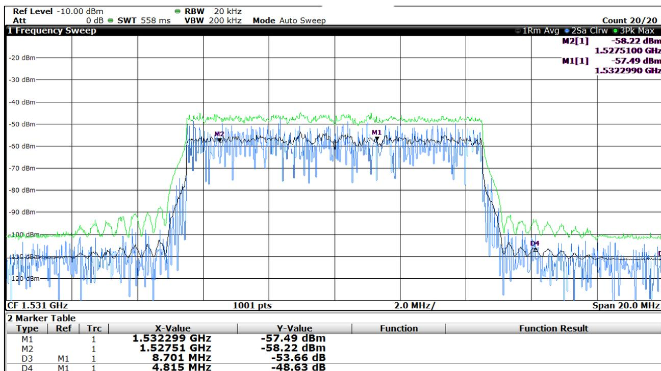
Figure H.6: E-TM3.2 signal, -33 dBm mean power
