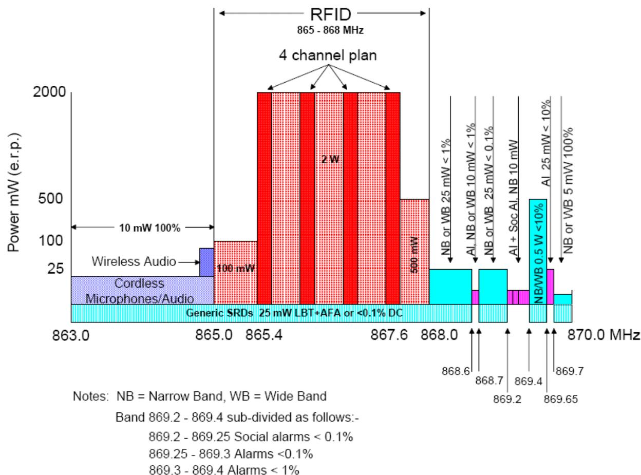
**Figure G.1: Short range Devices frequency plan according to the EC decision [i.3] related to Short Range Devices**
