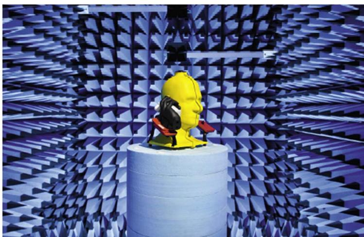
**Figure F.3: TRP test set up in an anechoic chamber**
