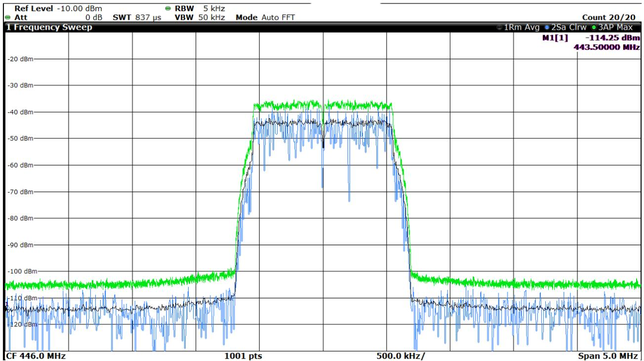
Figure H.9: 1,4 MHz LTE Signal E-TM2
