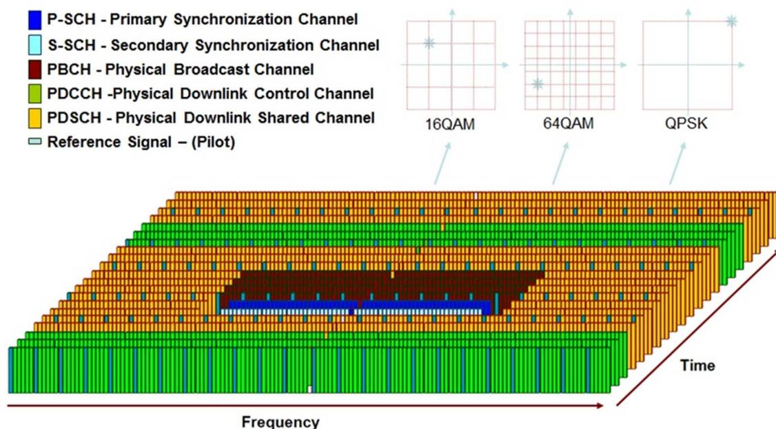
NOTE: The Y axis represents time (1 frame, i.e. 20 slots) and the X axis represents frequency, namely sub-carriers relative to the signal centre frequency (Source: Agilent Application Notes).
