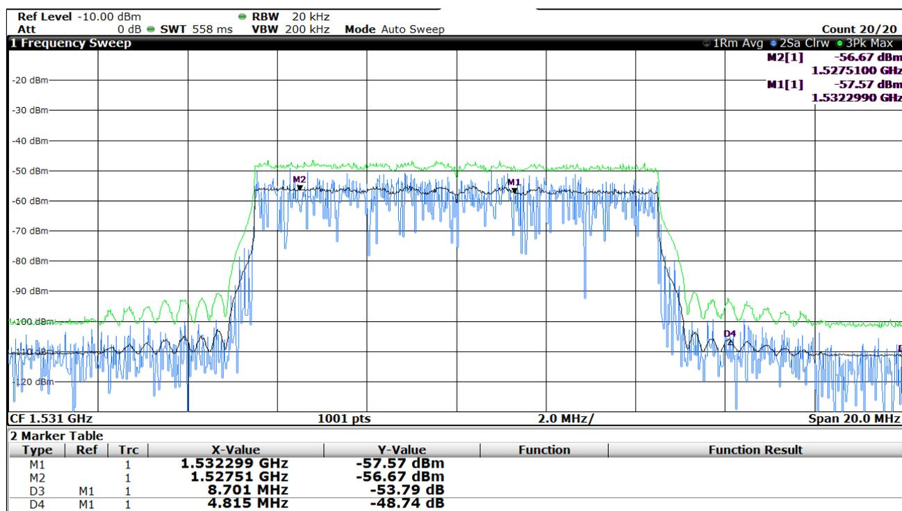
Figure H.5: E-TM3.1 signal, -33 dBm mean power
