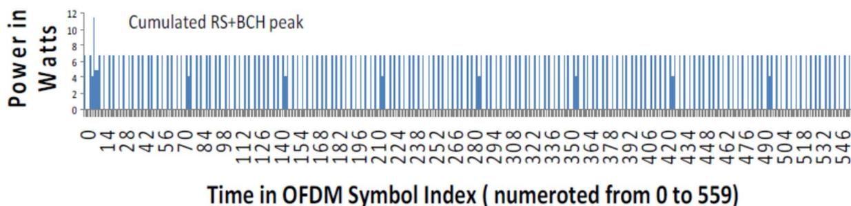
NOTE: This pattern is repeated every 40 ms. For a case when power is 2 x 40W the levels in this figure also doubles (Source: Orange).
