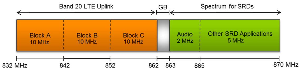
Figure 1: Spectrum allocation within 800 MHz
