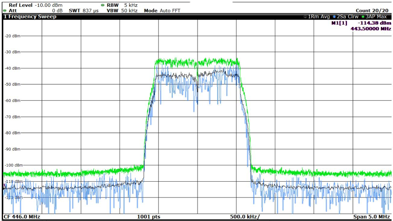
Figure H.11: 1,4 MHz LTE Signal E-TM3.2
