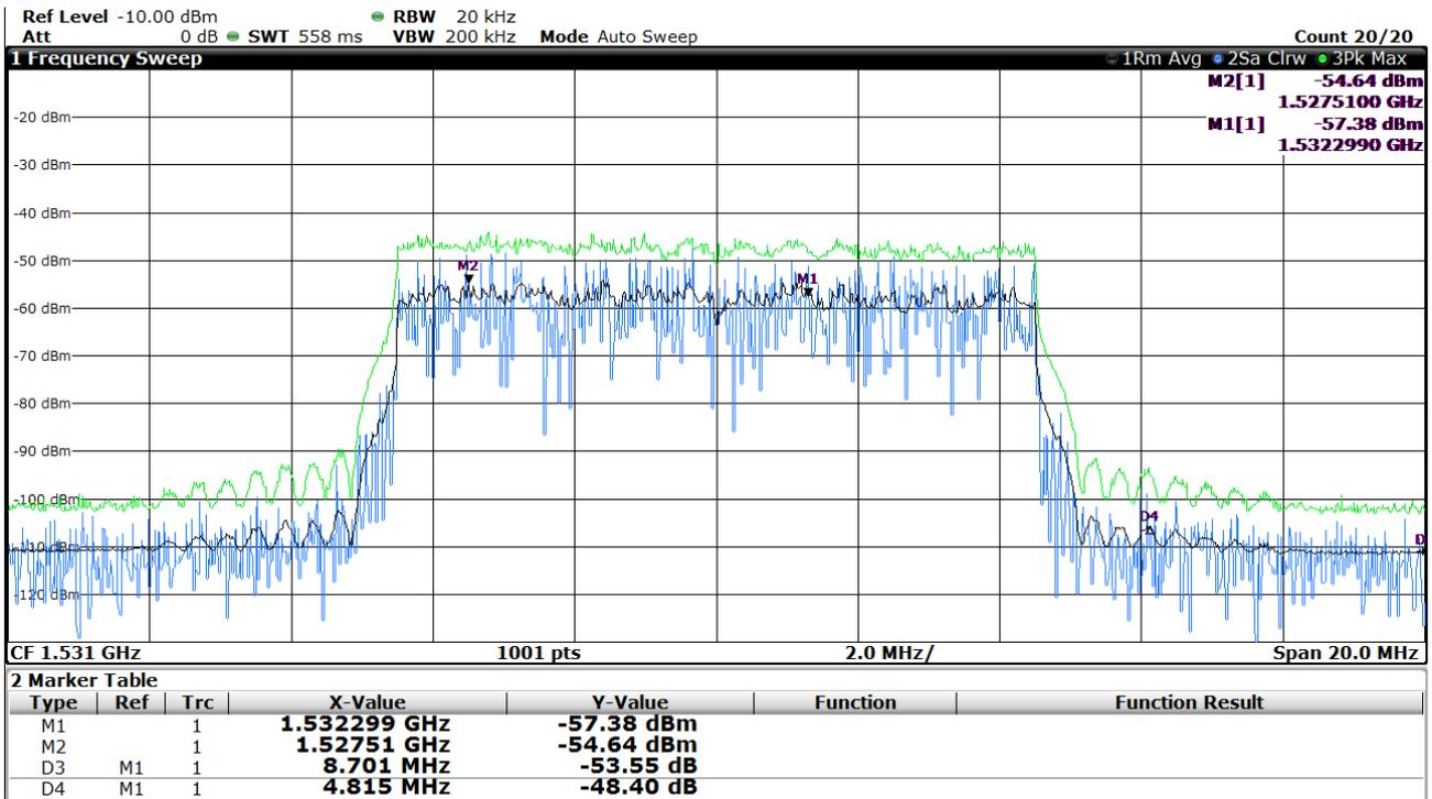
Figure H.2: E-TM1.2 signal, -33 dBm mean power
