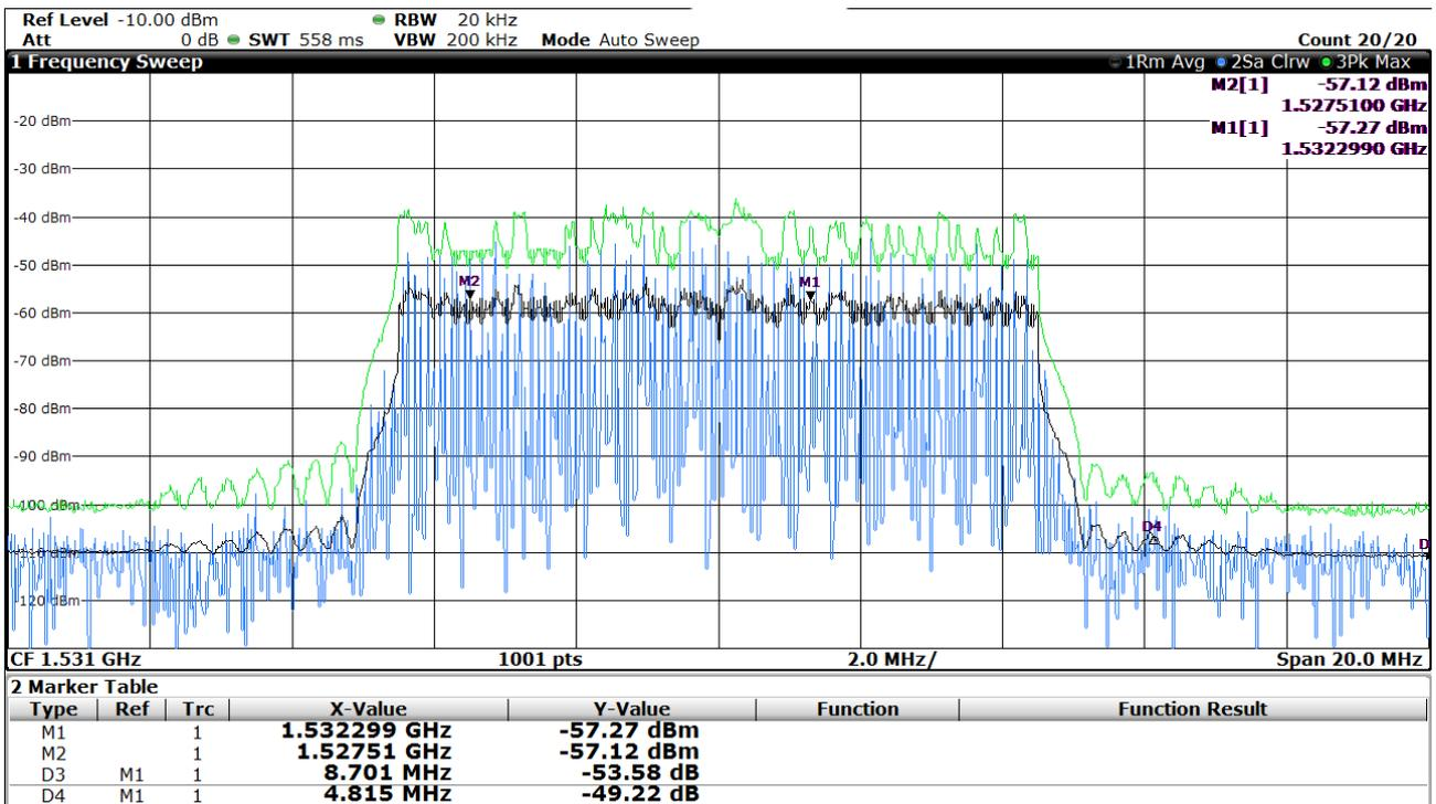
Figure H.3: E-TM2 signal ("idle mode"), -33 dBm mean power, Slow sweep
