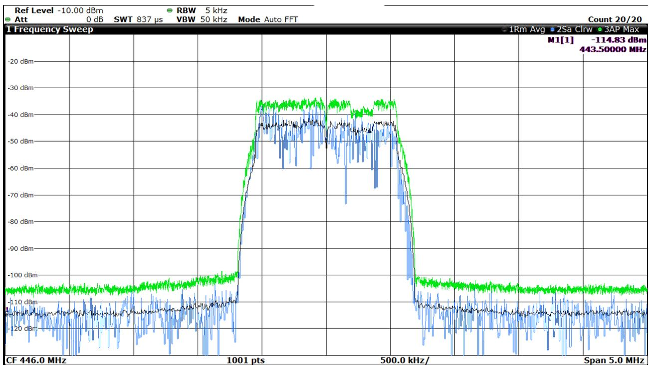
Figure H.8: 1,4 MHz LTE Signal E-TM1.2
