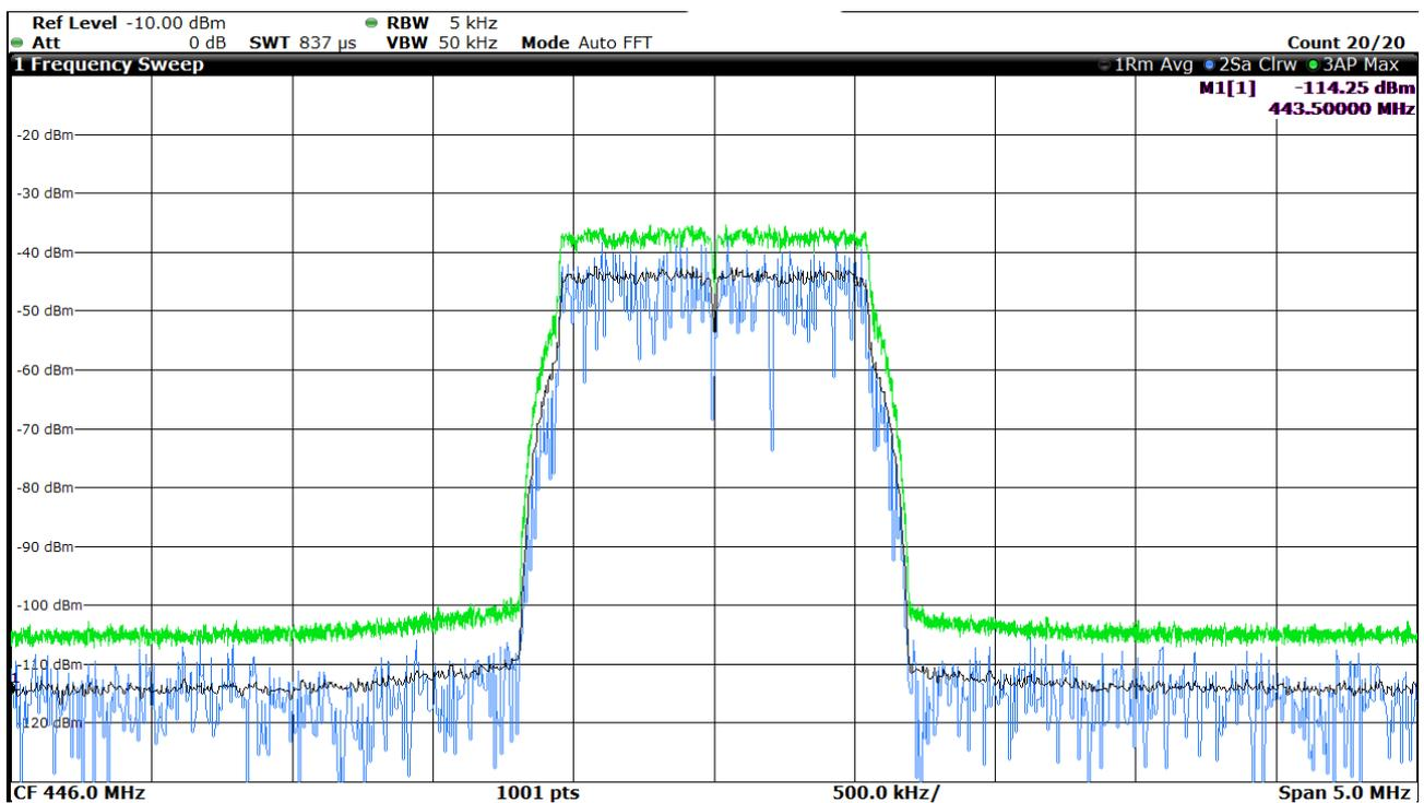
Figure H.10: 1,4 MHz LTE Signal E-TM3.1
