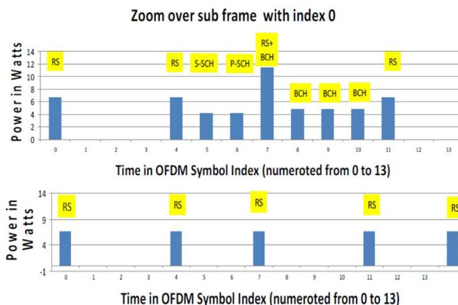
NOTE: BCH is repeated only every 4<sup>th</sup> frame. Synch signals are repeated every subframe. Rest of the subframes contain only RS signals (Source: Orange).
