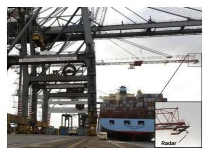
Figure B.19: Anti-collision system for Ship to Shore cranes (courtesy of Navtech Radar Ltd)
