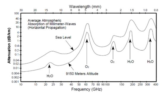
Figure 4: Atmospheric absorption of millimetre waves
