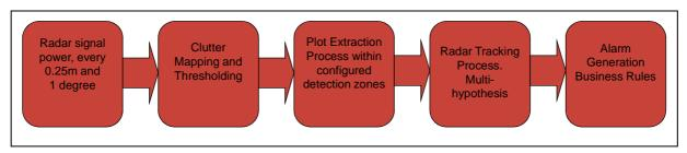
Figure A.1: Radar signal processing chain
