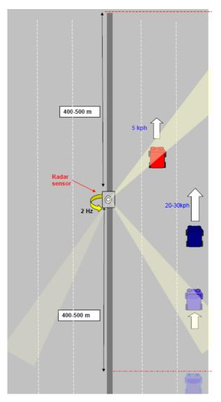
Figure C.4: Diagram showing radar scanning road
