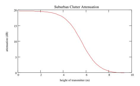
by 4 dB to A  $_{ht}(4 \cdot m) = 17.609$  dB and for 2 m by 6 dB to A  $_{ht}(2 \cdot m) = 19.506$  dB.
