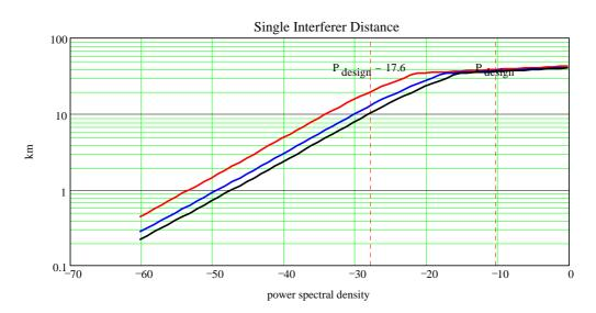
red: transmitter at 5 m above ground, blue, transmitter at 4 m above ground, black: transmitter 2 m above ground. without sector blanking  $_{d}$  <sub>SE</sub>  $(P_{design}) = _{38.64}$   $\cdot_{km}$ , for 4 m and 2 m, this does not change significantly:
