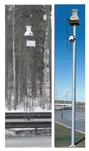
Figure C.3: Radar mounting posts (courtesy of Navtech Radar Ltd)
