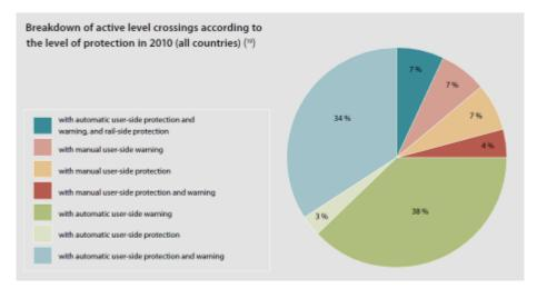
Figure B.12: Breakdown of active level crossings according to the level of protection in 2010, (source: Rail Safety and Standards Board)
