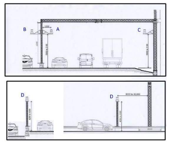
Figure C.1: Example radar sensor locations, (courtesy of Navtech Radar Ltd)
