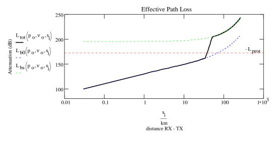
Separation distance:  $d_{min} := wurzel (L_{tot} (p_{o}, v_{o}, y) + L_{prot}, y) = d_{min} = 38.64 \cdot km$
