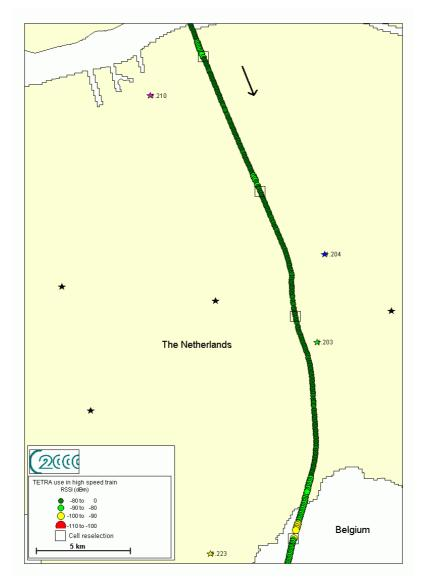
Figure 13: Received Signal Strength Indication (dBm)
