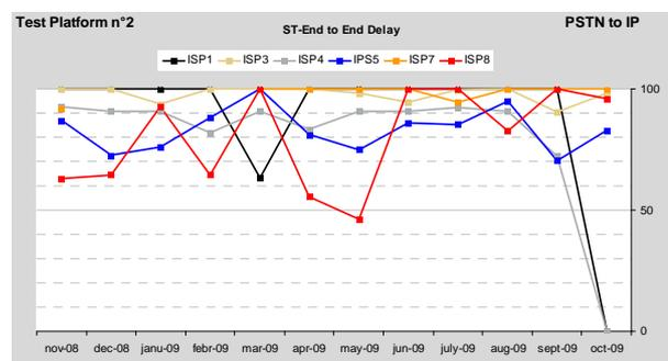
Concerning the variation of delay, we notice a relative consistency of the performances between all the offers. There is no offer with a very weak stability and there is no offer with a perfect stability (indicator value equal to 100 %) in both transmission directions, throughout the whole year. On the other hand two offers (ISP1 and ISP7) on platform N°2 present a perfect stability in IP to PSTN transmission direction.
