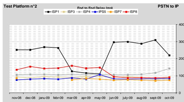
Concerning the end to end delay, we notice that in the PSTN to IP transmission direction, the delay is globally lower or close to 150 ms (on platforms N°1 and N°2).
