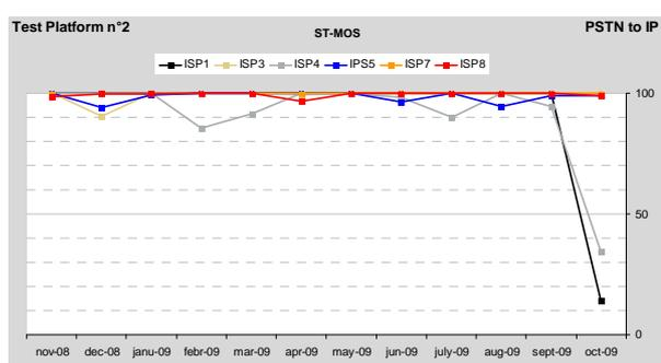
Concerning the speech quality, the stability is not bad. Except for the performances of the offer of ISP4 on platform N°2, in IP to PSTN transmission direction, the stability (according to transmission way) is characterized by mean values 99 % and 98 % on platform N°1 and by the mean values 94 % to 97 % on platform N°2. Hence normally we notice that the stability of speech quality is appreciably higher on the platform N°1.
