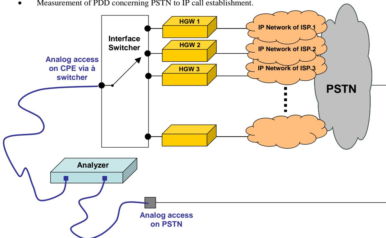
**Figure 1: Overview diagram of the measurement chain deployed on both platforms of follow-up**
