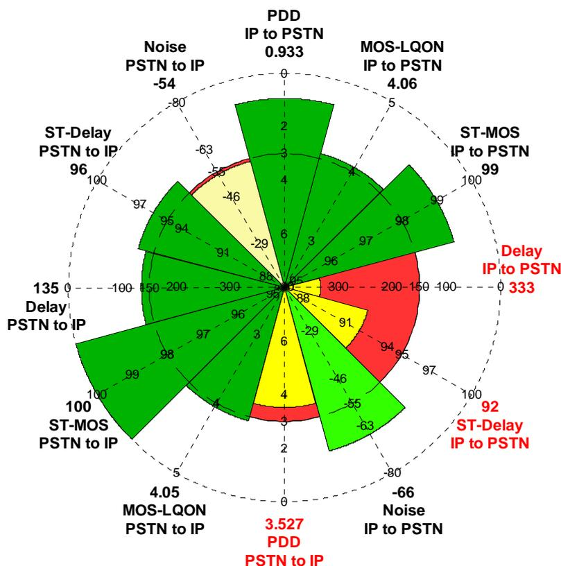
Figure 2: Example of Pie diagram with indicators determined within the framework of the two platforms of the VoIP offers
