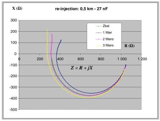
Figure B.6: Impedances presented at the FXS port, comparison with new balance impedance Z<sub>bal</sub> - 0,5 km local loop
