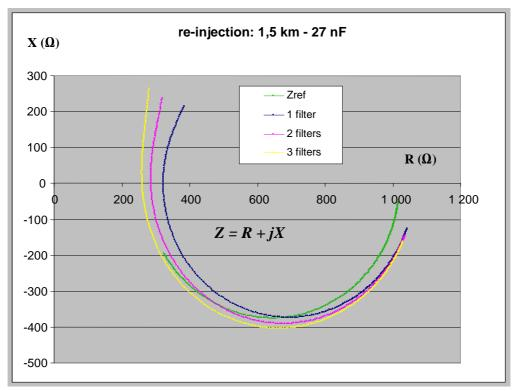
Figure B.11: Impedances presented at the TE port for FXS=Z<sub>R</sub> - 1,5 km local loop
