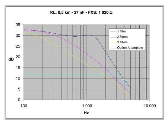
Figure B.14: Return Loss (with respect to  $Z_R$ ) of impedances presented at the TE port (FXS = 1 020  $\Omega$ ) - 0,5 km local loop
