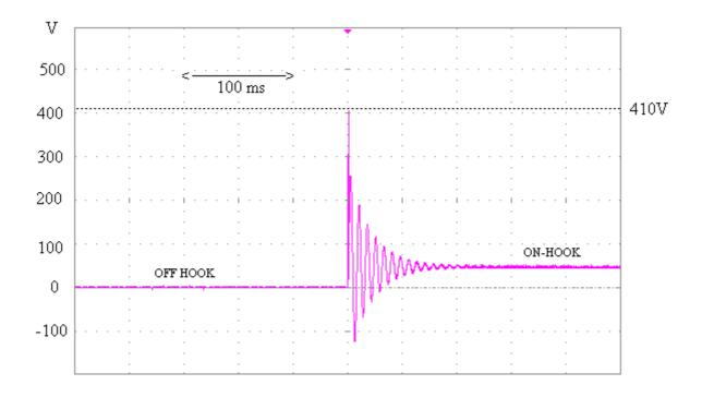
Figure 28: On/off-Hook transients. Re-injection scenario. One microfilter.
