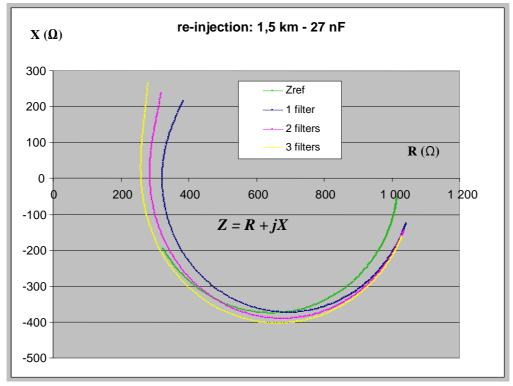
Figure B.2: Impedances presented at the FXS port - 1,5 km local loop
