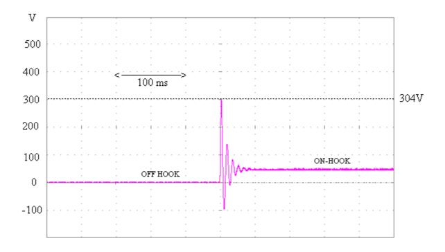
Figure 26: Off/on-Hook transients. Traditional xDSL deployment. Two microfilters.
