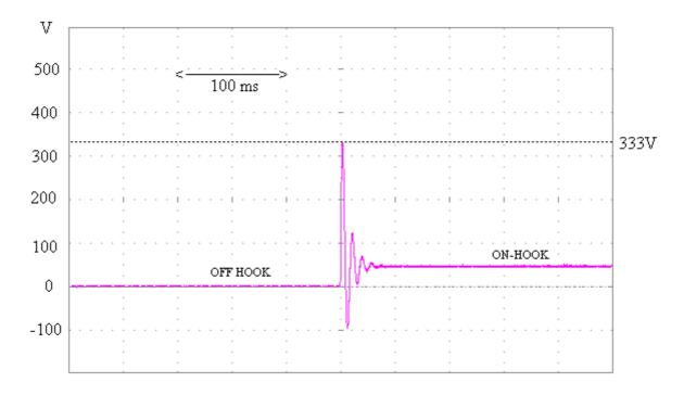
Figure 30: On/off-Hook transients. Re-injection scenario. Three microfilters.
