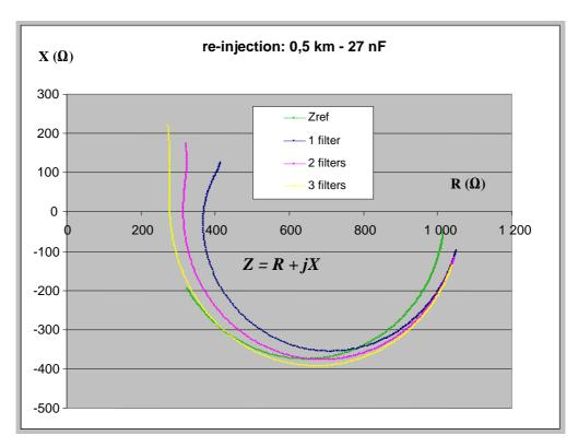
Figure B.10: Impedances presented at the TE port for FXS=Z<sub>R</sub> - 0,5 km local loop
