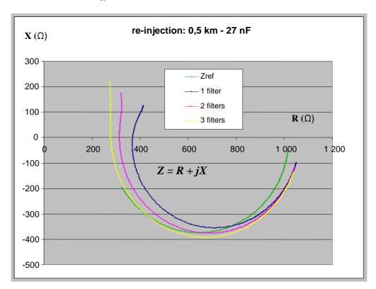
Figure B.1: Impedances presented at the FXS port - 0,5 km local loop
