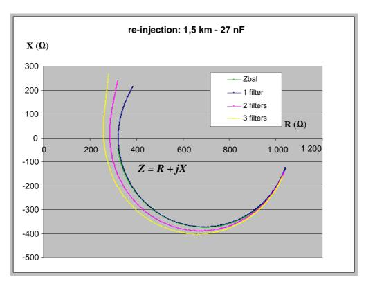
Figure B.7: Impedances presented at the FXS port, comparison with new balance impedance  $Z_{bal}$  - 1,5 km local loop
