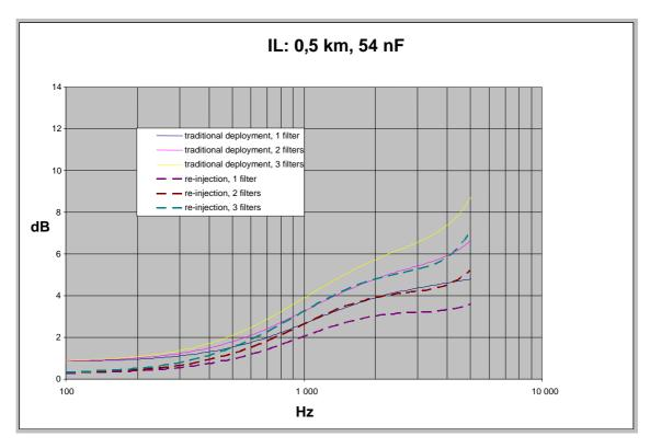
NOTE Cable length: 0,5 km. High capacity microfilters.
