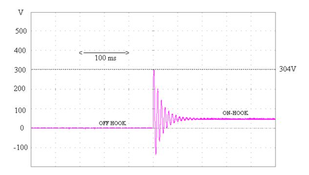
Figure 25: Off/on-Hook transients. Traditional xDSL deployment. One microfilter.
