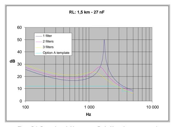
Figure B.9: Return Loss (with respect to  $Z_{bal}$ ) of impedances presented at the FXS port - 1,5 km local loop
