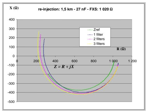
Figure B.13: Impedances presented at the TE port for FXS=1 020  $\Omega$  - 1,5 km local loop
