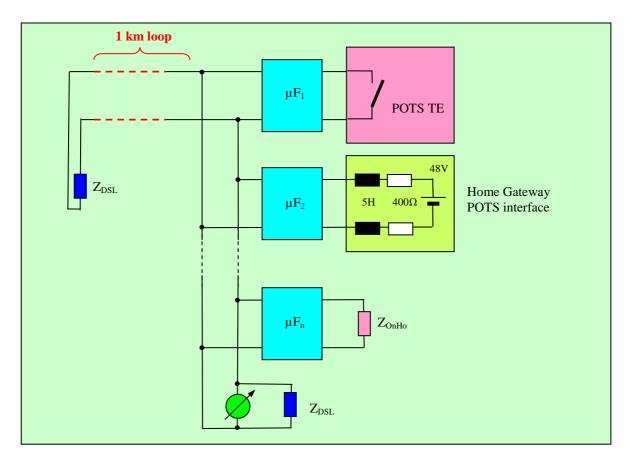
Figure 24: test of the on-hook/off-hook transients at the xDSL interface of the HG for the re-injection scenario
