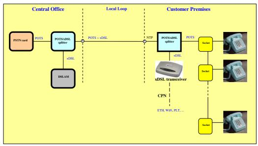
Figure 1: Telephony and xDSL deployment from the CO - centralised splitter
