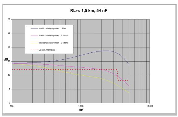
NOTE: Cable length: 1,5 km. High capacity microfilters.
