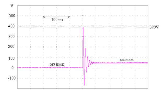
Figure 28: On/off-Hook transients. Re-injection scenario. Two microfilters.
