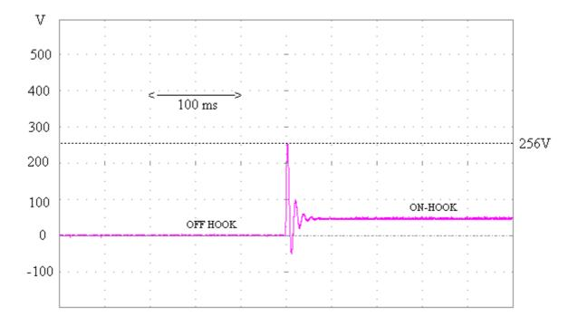
Figure 27: On-Hook transient. Traditional xDSL deployment. Three microfilters.
