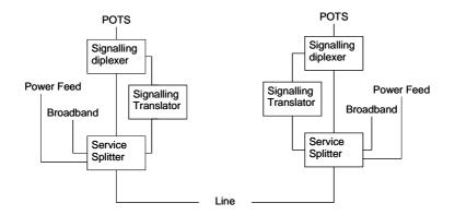
Figure 13: Analogue port replicator sub-system (POTS Adapter)
