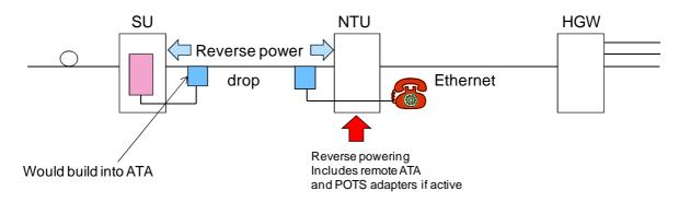
Figure 19: ATA In Service Unit (SU) With POTS Adaptors
