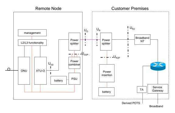
Figure 16: Derived POTS Solution
