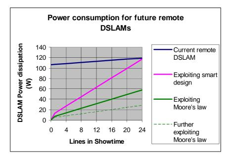
Figure 9: Power Consumption for Future Remote DSLAMS
