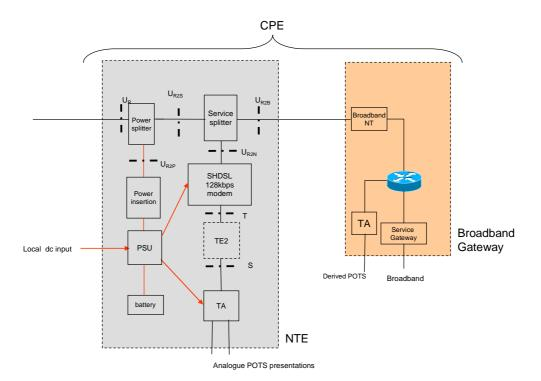
Figure 15: Baseband POTS Delivery via Channelised SHDSL
