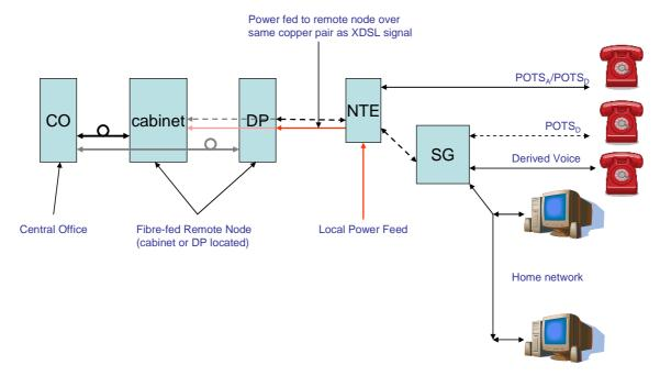
Figure 1: Generic Reverse Power Feed Architecture
