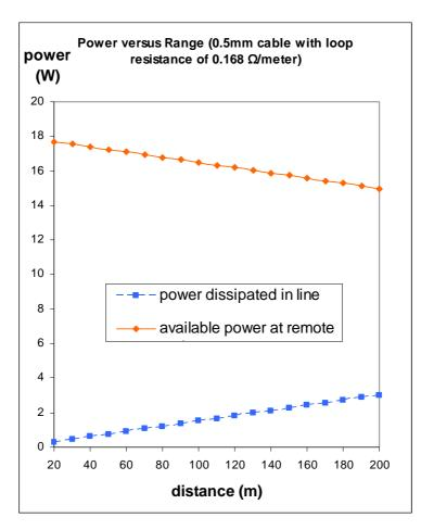
Figure 10: Range versus Power for Reverse Power Feed (60 V@300 mA)
