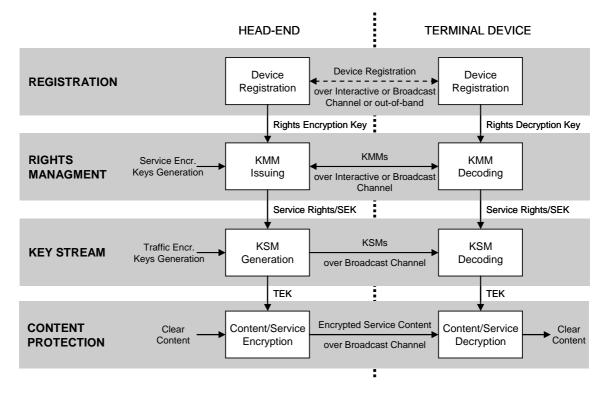
Figure 13: Hierarchical Model for Service Protection
