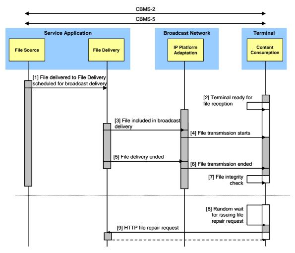
Figure 12: Message flow for File Delivery
