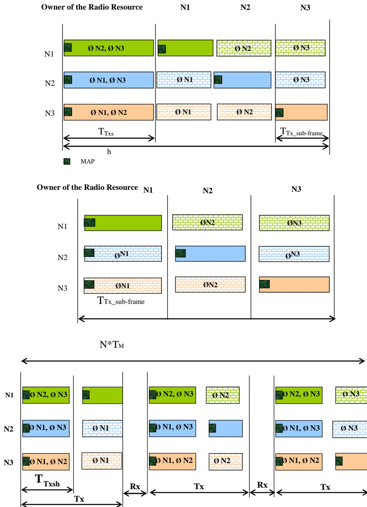
**Figure C.2: Power control and traffic scheduling with a Coexistence Protocol**
