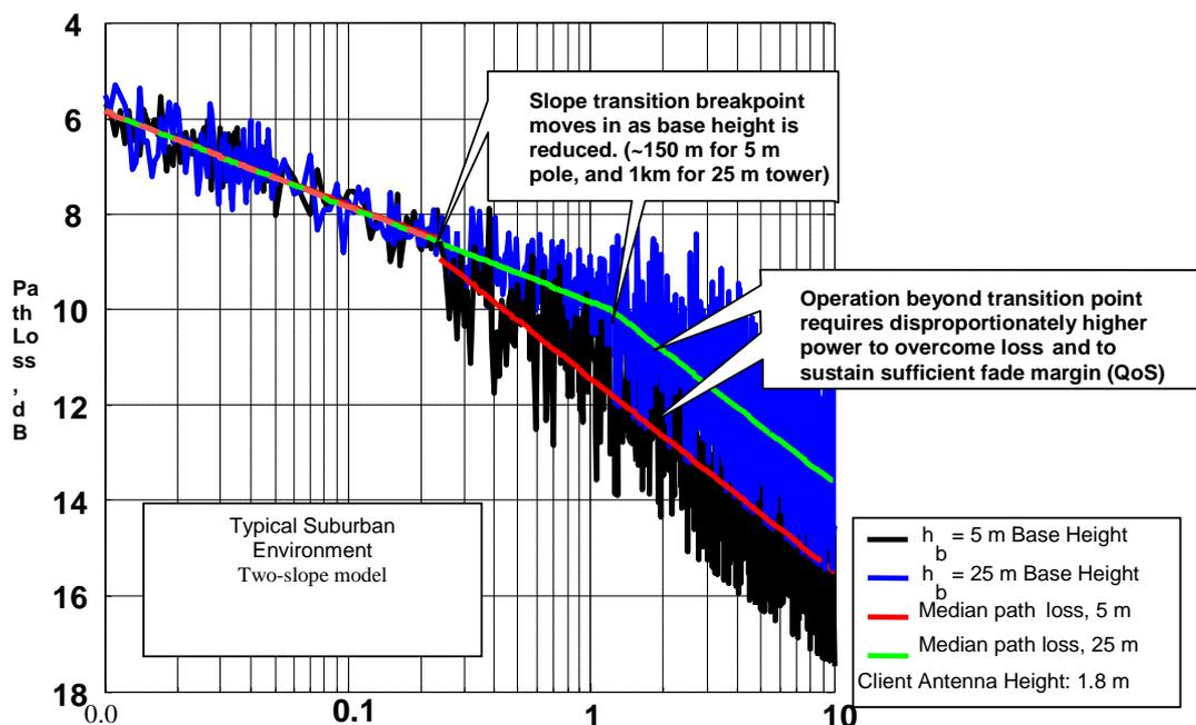
Figure B.10: Measured path loss at 2.4 GHz
