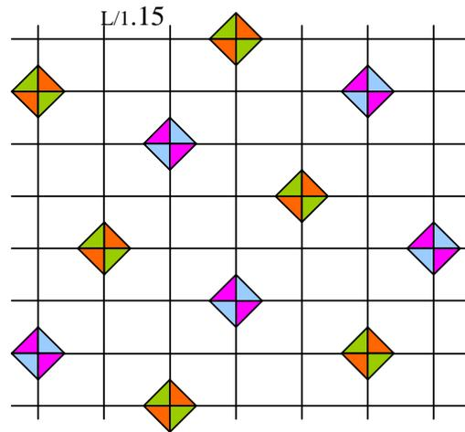
Figure B.7: Example 2 of frequency distribution, reuse factor = 2
