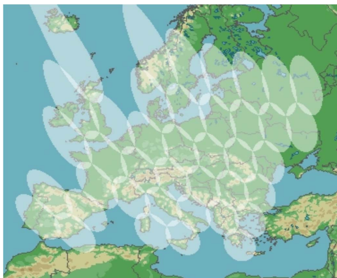
Figure D.1: 40 Ka-band spot beams spread over a typical European coverage
