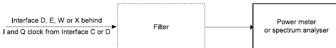
Figure E-14: Test set-up for out-of-service noise power measurement
