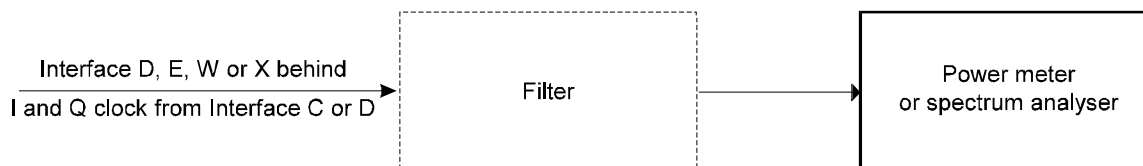
Figure E-13: Test set-up for RF/IF power measurement
