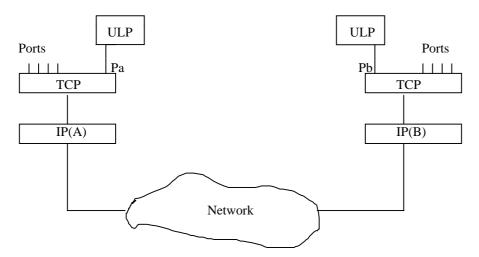
Figure 4: TCP connection structure
